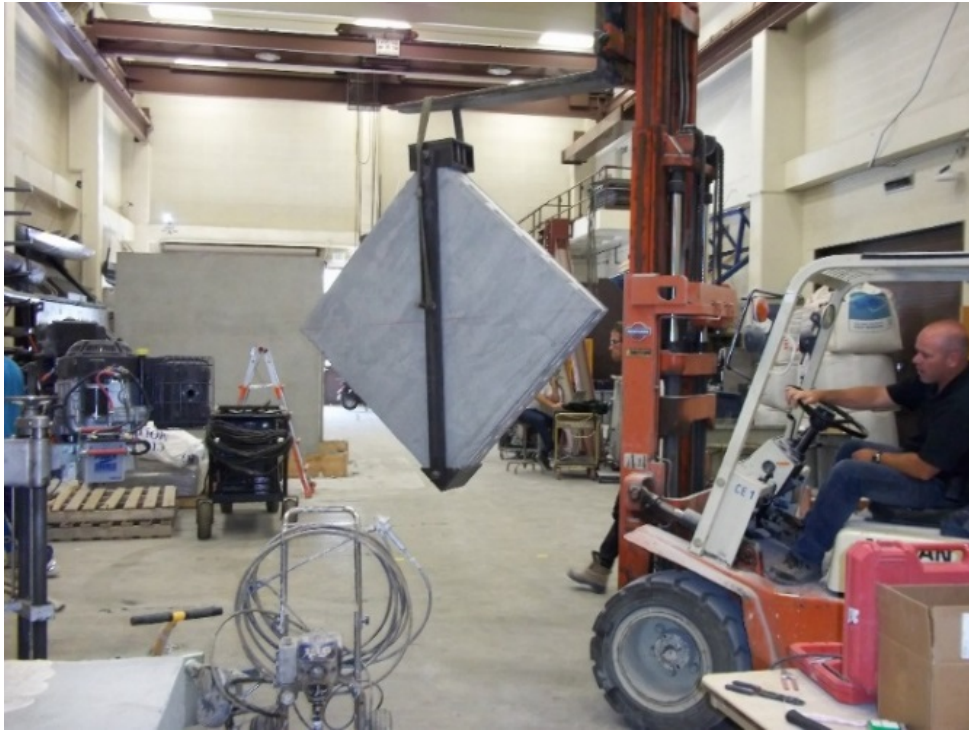
Figure 3-14 Transportation of walls during diagonal-tension test.
