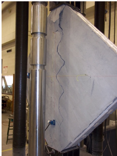
(a) Cracking of face of wallette.
