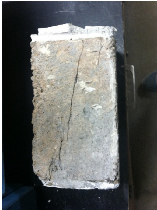
Figure 3-5 Typical failure of grout prisms.
