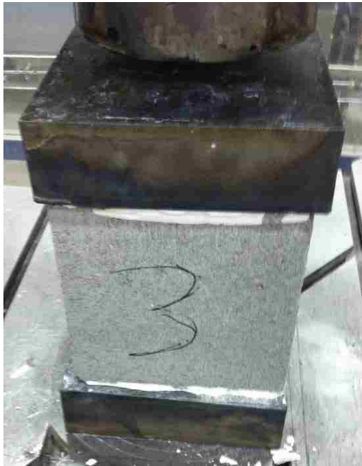
Figure 3-10 Block specimen being tested.
