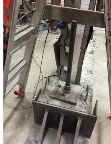
(c) Cracks in outer webs.
