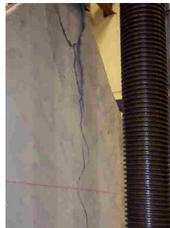
(a) Crack in block prior to testing. (b) Cracks in web after testing. (c) Crack on face.
