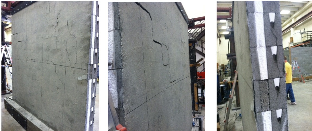
(a) Diagonal cracks. (b) Large shear crack opening. (c) Cracking of outside web.
