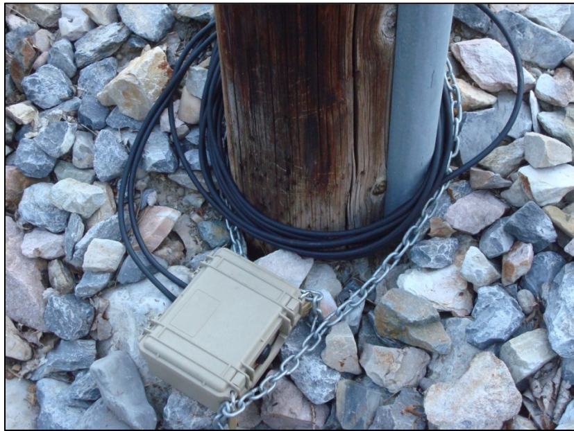
Figure 4-6: Placement of Trax Cycles Plus unit (photo taken by Chris Haskell, 2015).
