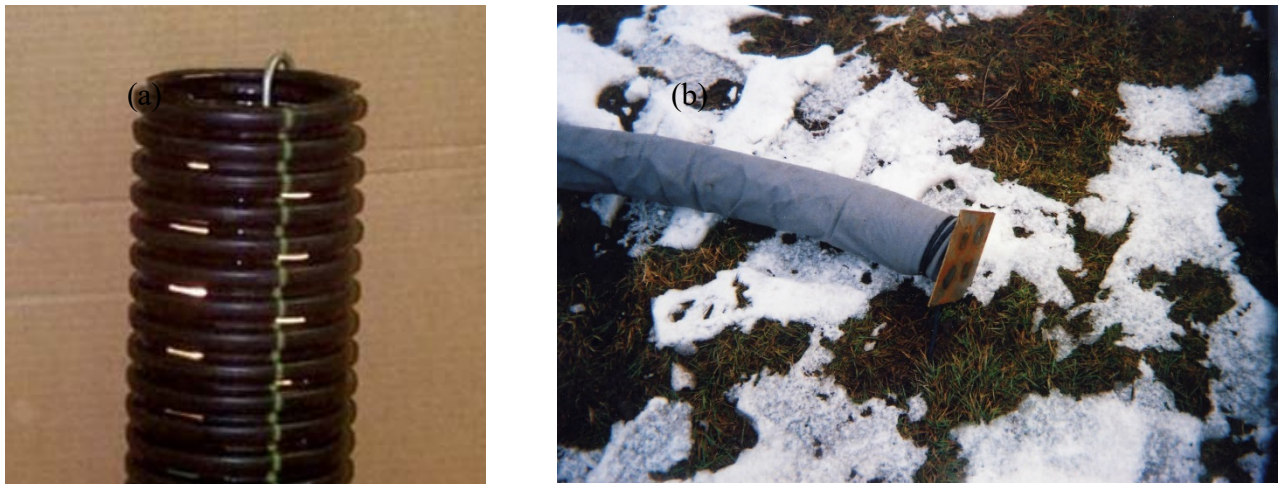
Figure 2 (a) EQ Drain Without Filter Fabric Showing Slots Illuminated by Light Inside Pipe and (b) EQ Drain with Filter Fabric and Anchor Plate at the End (Rollins et al, 2004).
