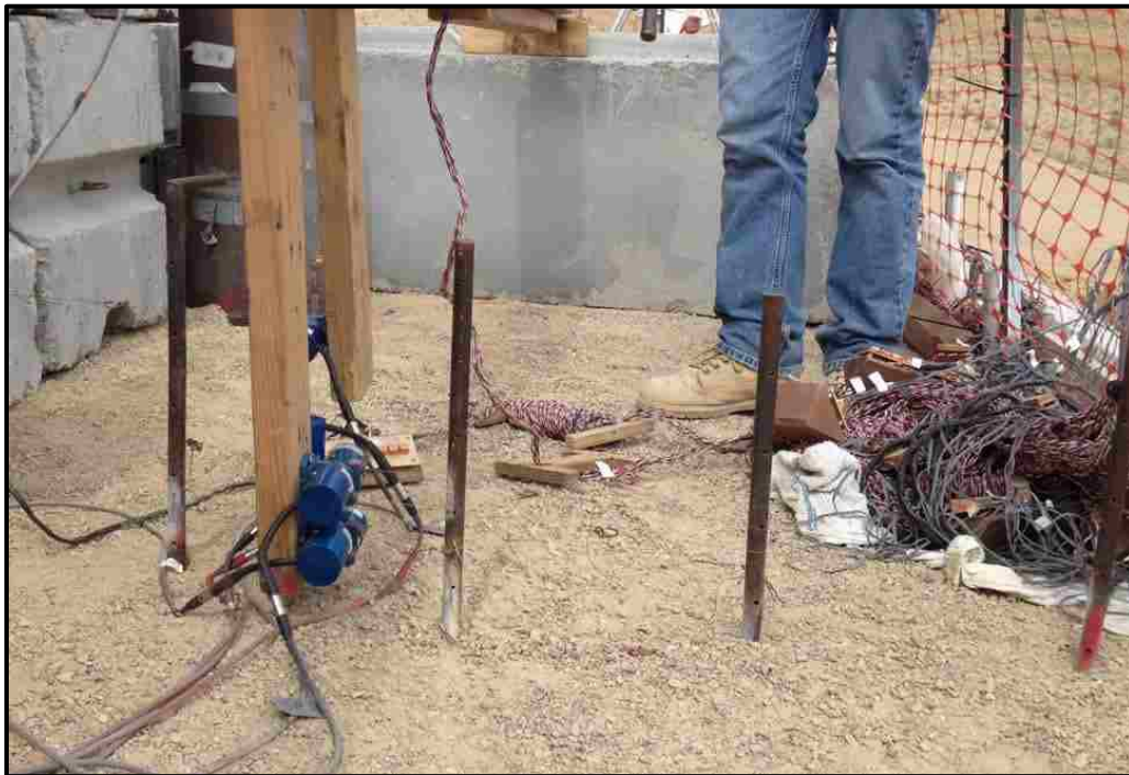
Figure 4-2: Horizontal ground displacement setup.
