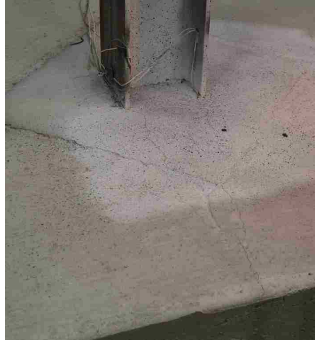
Figure 4-8: Specimen A1 at 0.04 Drift
