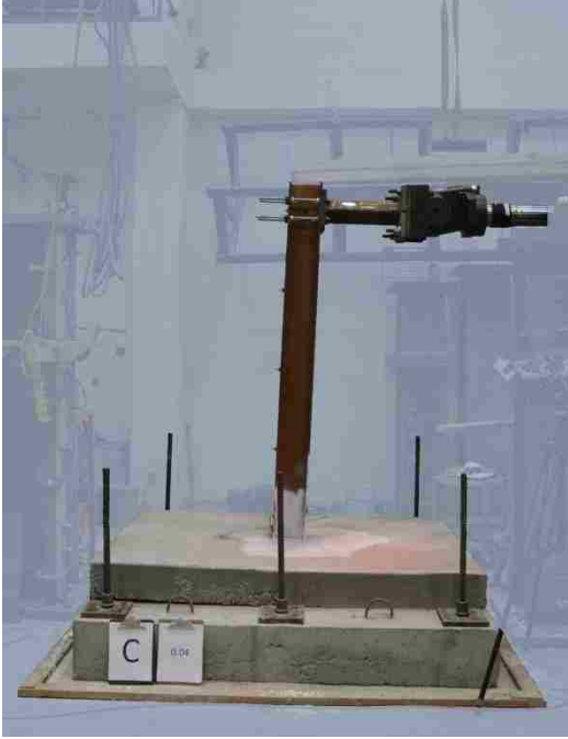
Figure 4-8: Specimen A1 at 0.04 Drift
