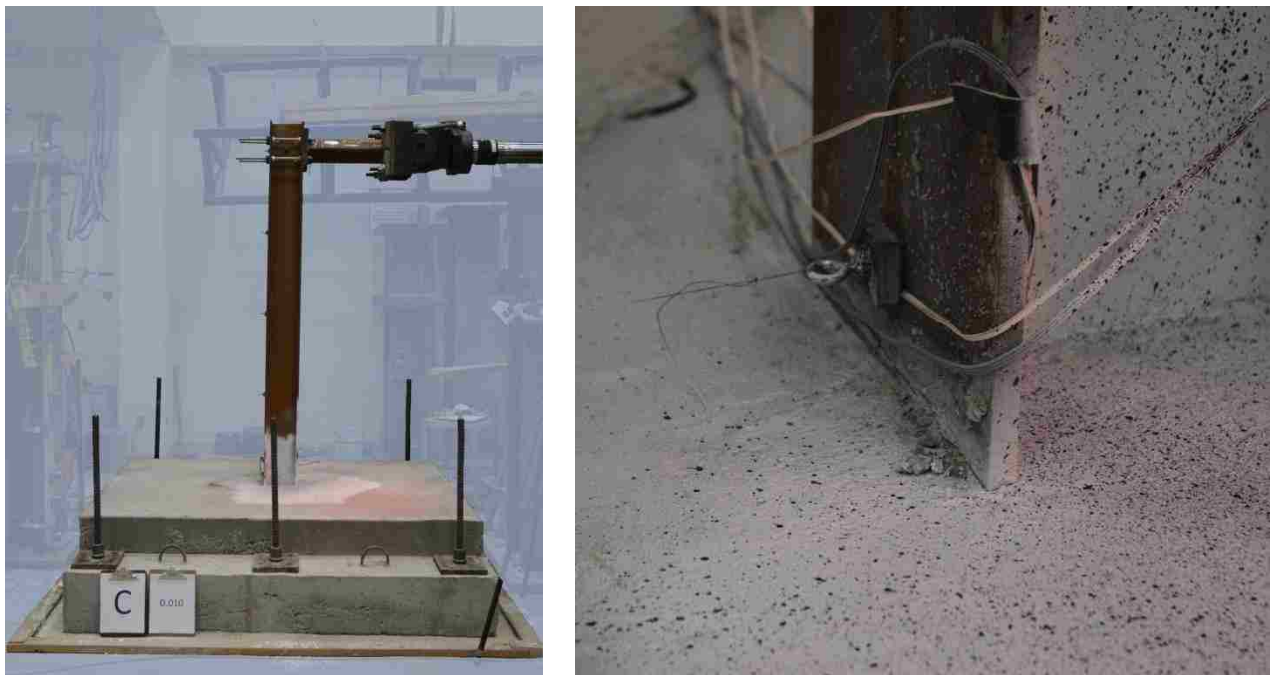
Figure 4-5: Specimen A1 at 0.01 Drift
