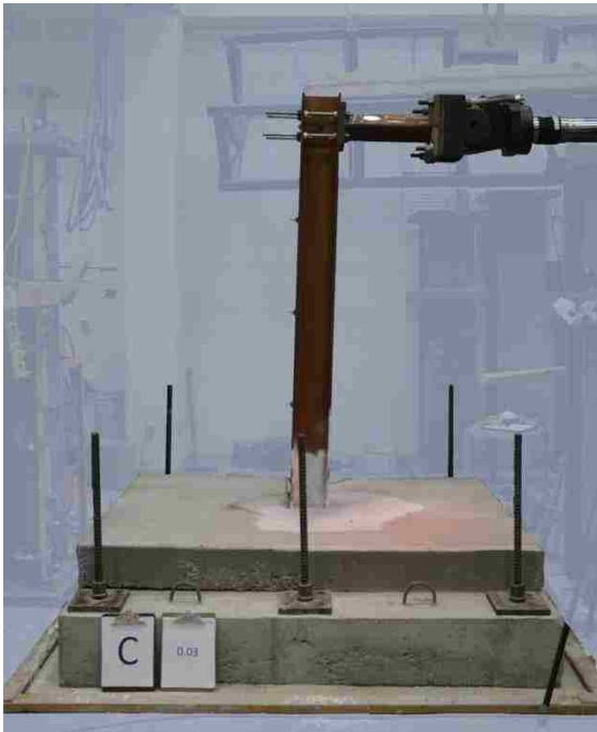
Figure 4-7: Specimen A1 at 0.03 Drift
