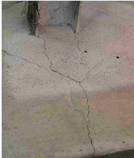
Figure 4-9: Specimen A1 at 0.05 Drift
