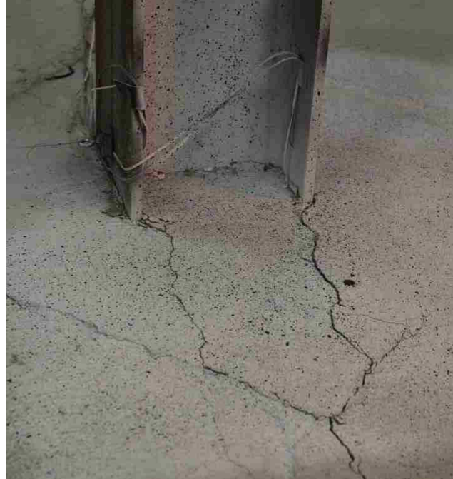
Figure 4-10: Specimen A1 at 0.06 Drift
