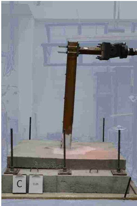
Figure 4-9: Specimen A1 at 0.05 Drift
