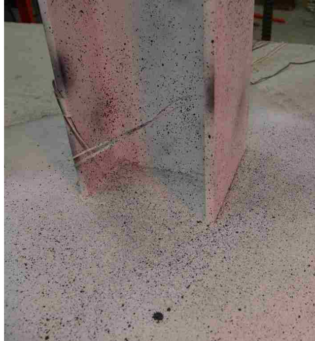
Figure 4-6: Specimen A1 at 0.02 Drift
