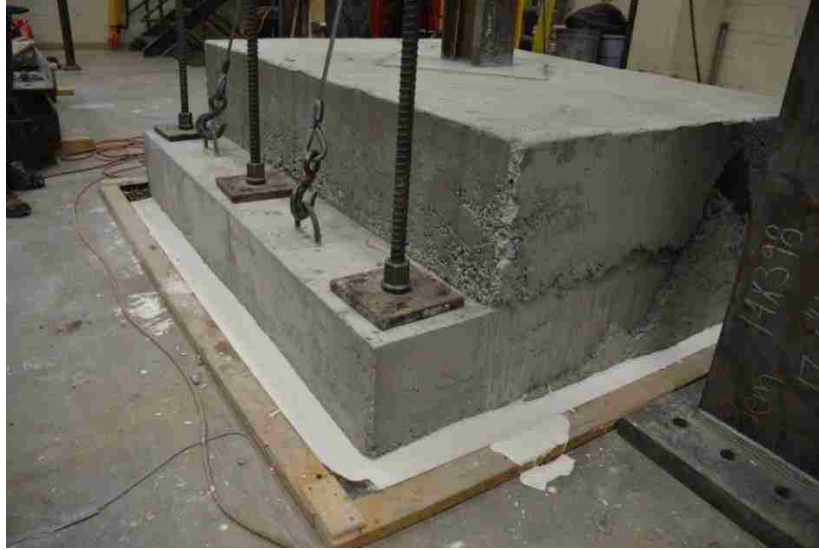
Figure 3-26: Specimen Immediately after Being Placed in HYDROCAL
