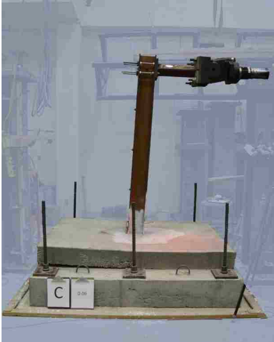
Figure 4-10: Specimen A1 at 0.06 Drift
