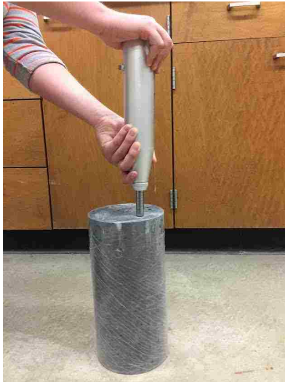
Figure 3-18: Schmidt rebound hammer testing.
