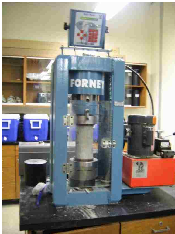
Figure 3-15: Compressive strength testing.
