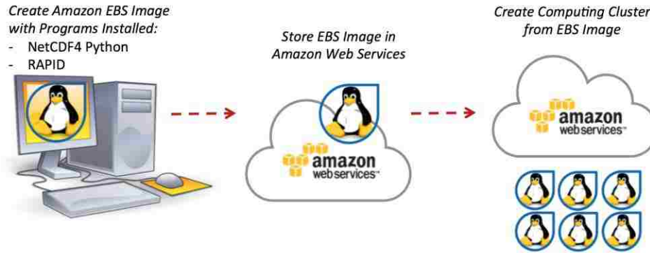
Figure 3-6 Diagram of Creating and Using EBS Image
