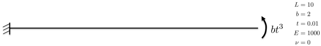
Figure 1.3: The cantilever beam.
