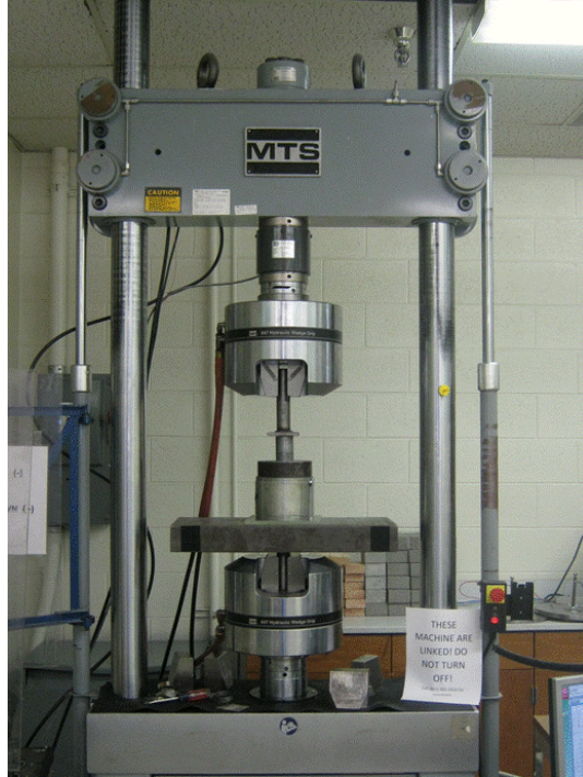
Figure 3-9: CBR specimen placed inside the Instron material testing machine.
