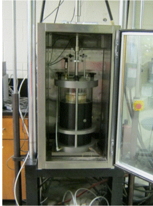
Figure 3-8: Triaxial cell placed inside the UTM-100.
