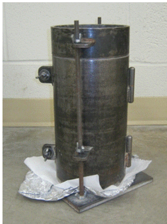
Figure 3-6: Steel split mold for compacting specimens.
