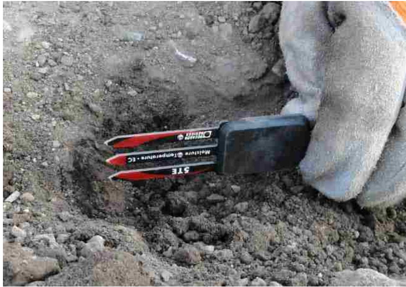
Figure 3-4: Soil moisture, temperature, and electrical conductivity sensor.
