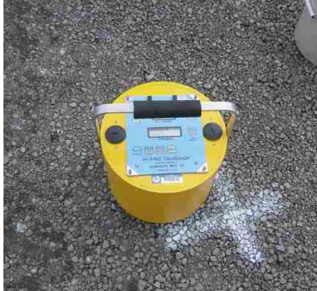
Figure 3-16: SSG testing of base layer.
