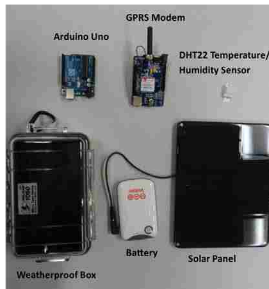
Figure 2. Arduino, solar panel, battery, sensor, and GPRS modem
