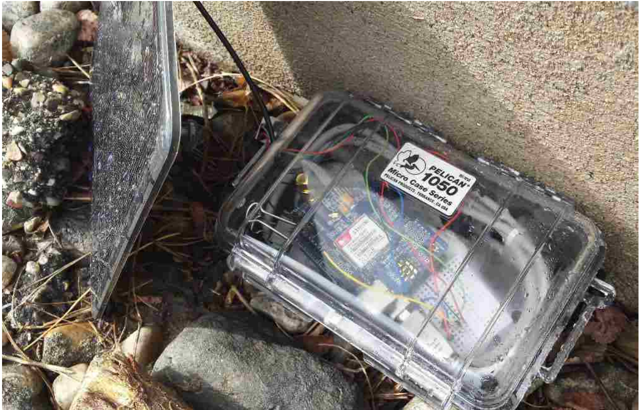
Figure 6. Sensor in first deployment location. The temperature sensor, not visible here, is external to the case.
