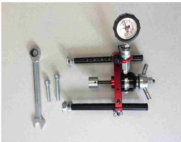
Figure 3-10: Helix Pullout Device
