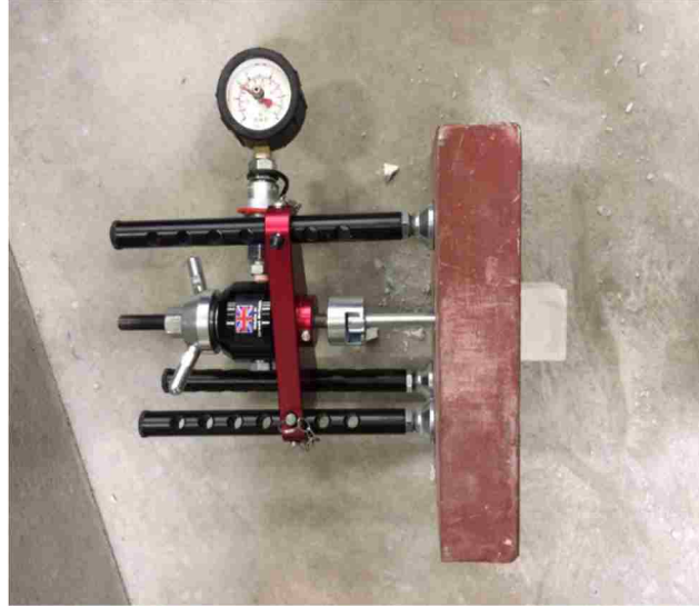
Figure 3-11: Helix Cube Test Setup
