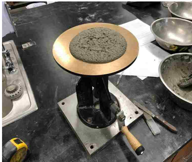
Figure 3-1: Mortar Flow Test
