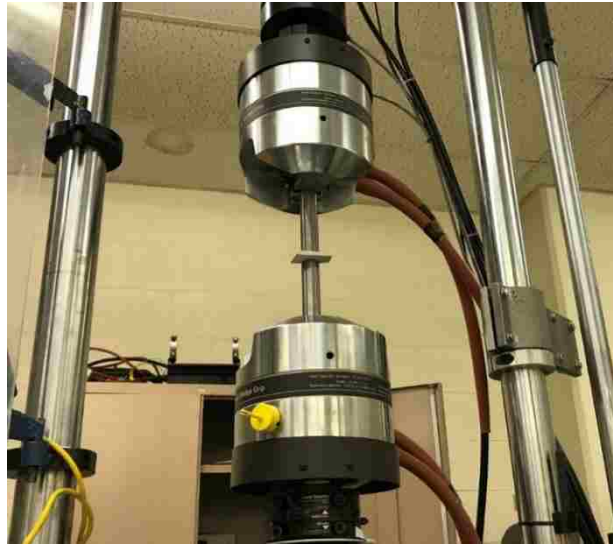
Figure 3-7: Double Punch Test Setup
