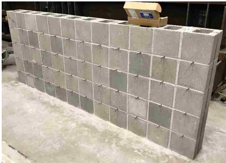
Figure 3-2: Wall Panel with Helical Ties
