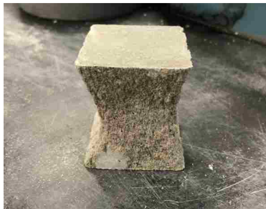
Figure 3-4: Mortar Cube After Compression Testing
