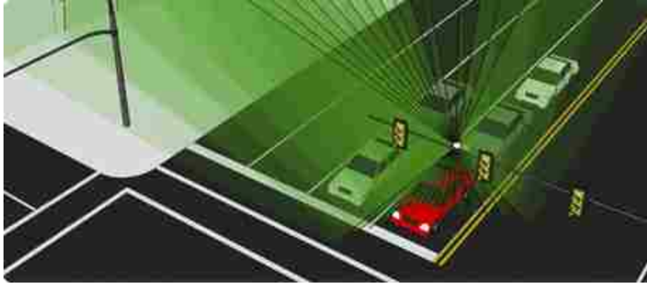
Figure 2-2: Vertical Beam Width (Wavetronix 2015a)
