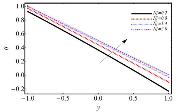
Fig. 8b. Effect of  $N_j$  on temperature profile.
