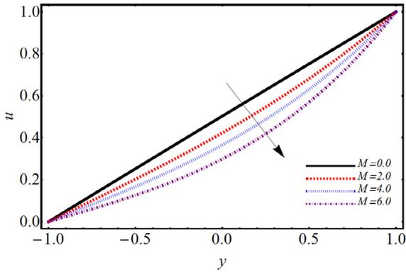
**Fig. 3a.** Effect of  $M$  on velocity profile.
