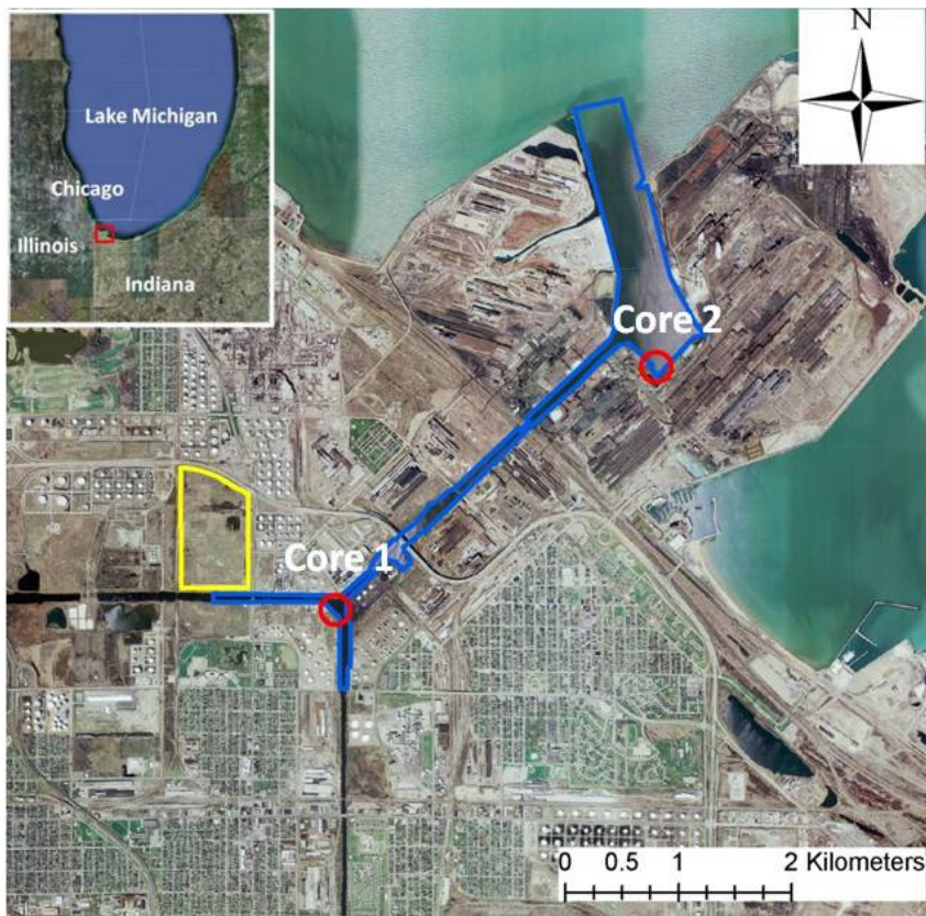
Figure 4-1 Indiana Harbor and Ship Canal, East Chicago, Indiana. Red circles show the core sample locations (Core 1: latitude 41^{\circ} 38.7425 N and longitude 87^{\circ} 28.3277 W, Core 2: latitude 41^{\circ} 39.9058 N and longitude 87^{\circ} 26.2944 W). The blue and yellow polygons represent the dredging area and the confined disposal facility (CDF), respectively (17)
