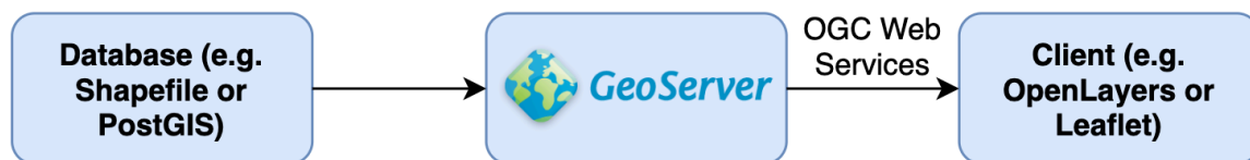
Figure 2-8: A diagram of GeoServer in a typical web app stack.
