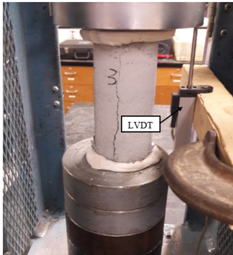
Figure 4-5: Cellular concrete cylinder after failure in UCS testing.
