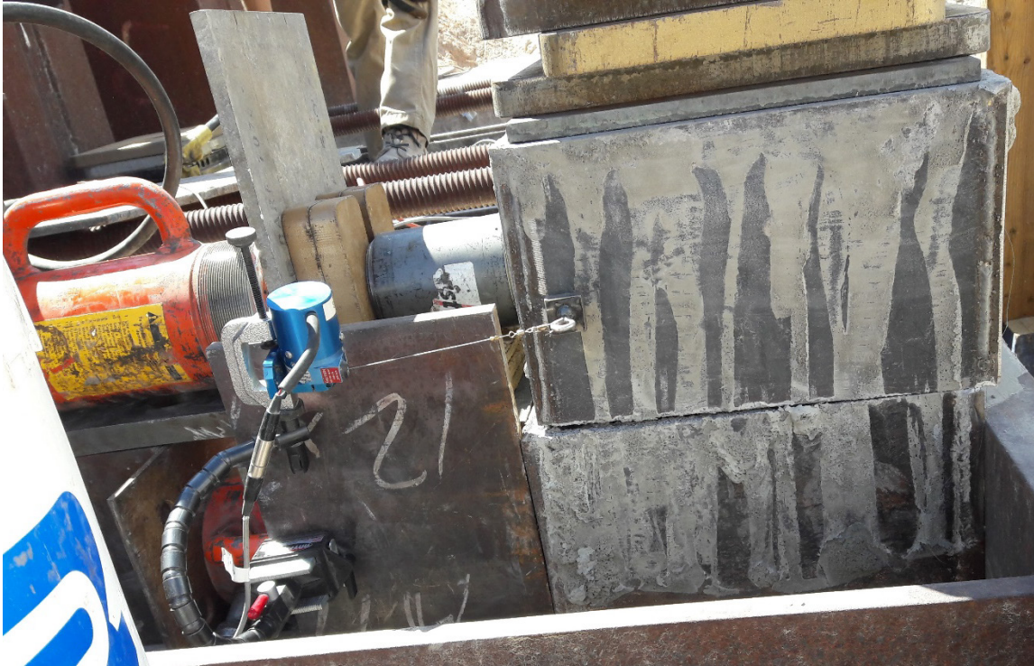
Figure 4-21: Rotation of upper box owing to applied moment during shear test.
