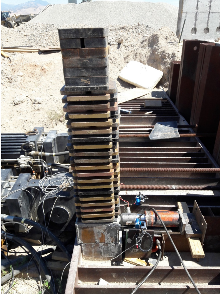
Figure 4-20: Direct shear test for cellular concrete with normal load of 1,799 lb (816 kg).
