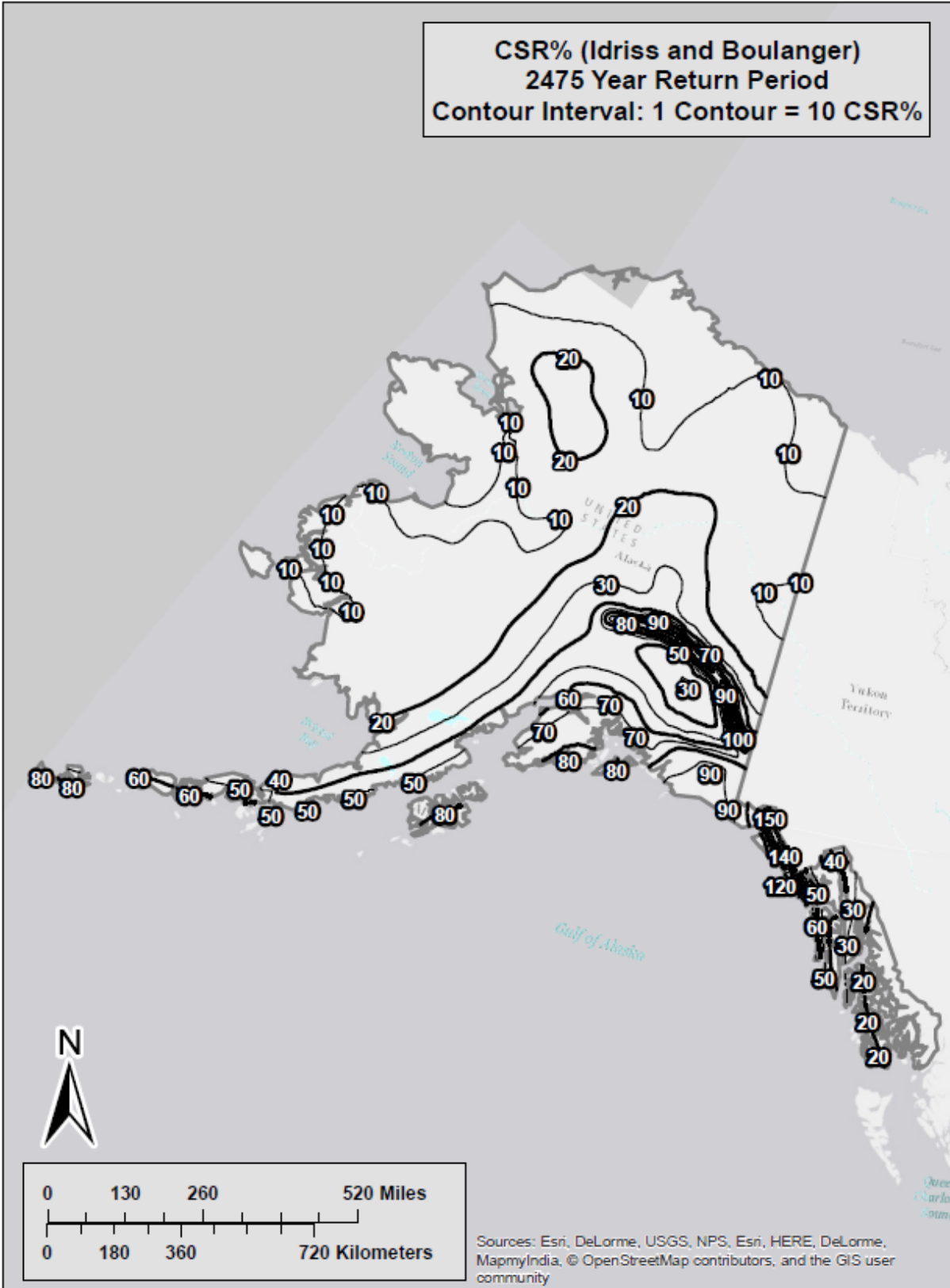
Figure B-5 Liquefaction Triggering ( CSR\%_{ref} ) Map for Alaska ( T_r = 2,475 )
