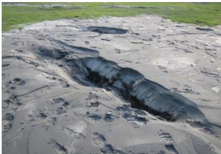
Figure 2-14: Large Sand Boil after the Darfield, 2010 Event (courtesy of GEER, 2010)
