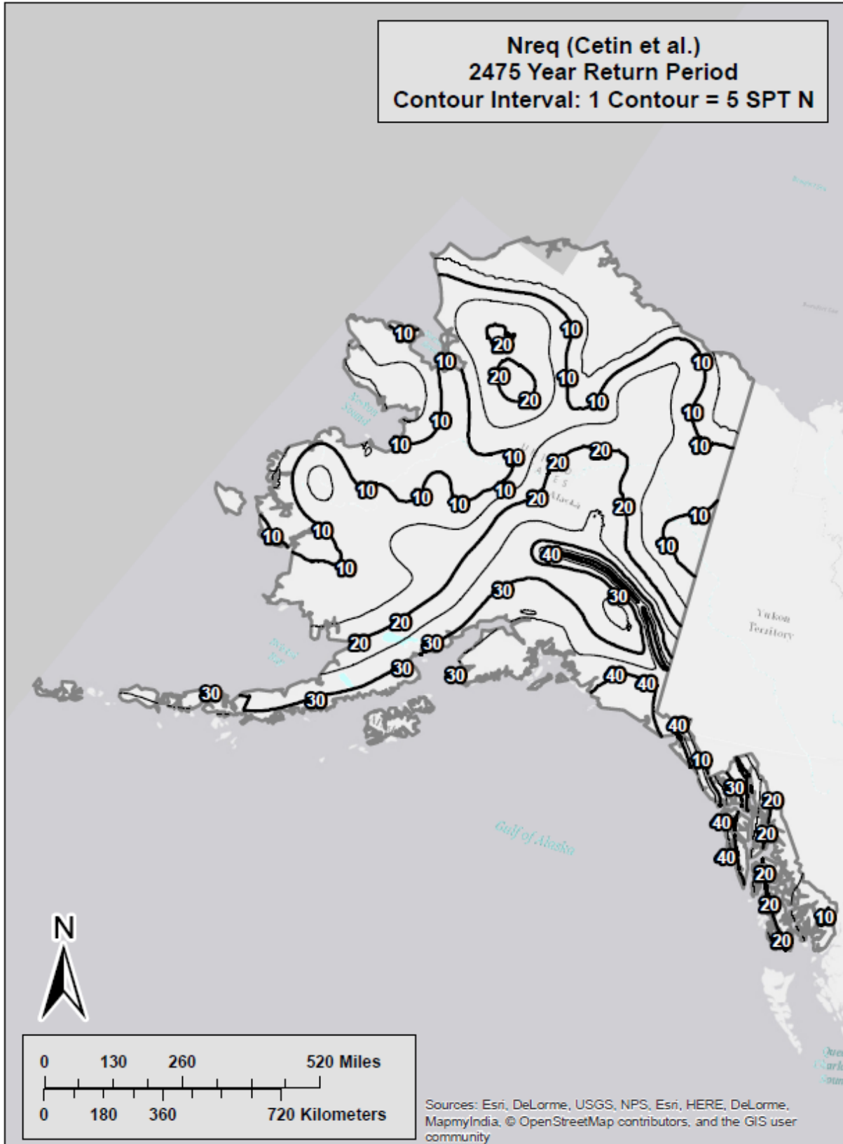
Figure B-6 Liquefaction Triggering ( N_{req}^{ref} ) Map for Alaska ( T_r = 2,475 )
