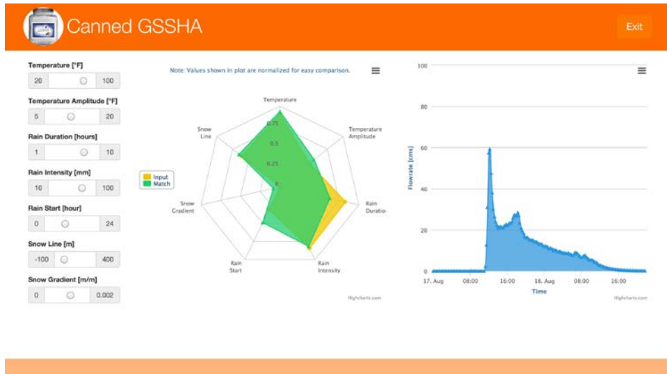
Figure 4-1. A screenshot of the Canned GSSHA web app developed using Tethys Platform.
