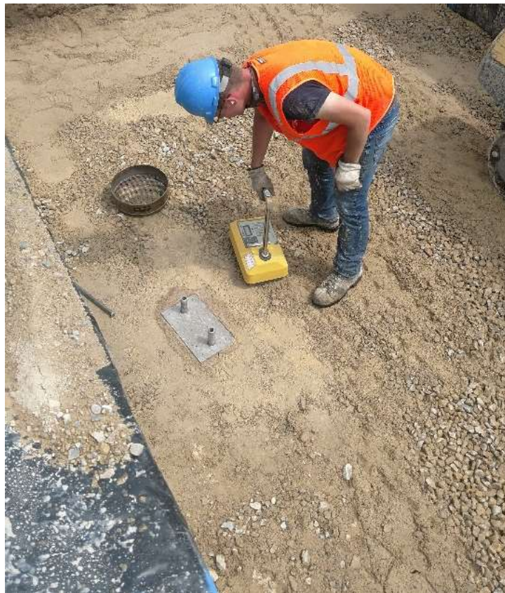
Figure 3-12. The author performing a nuclear density test.
