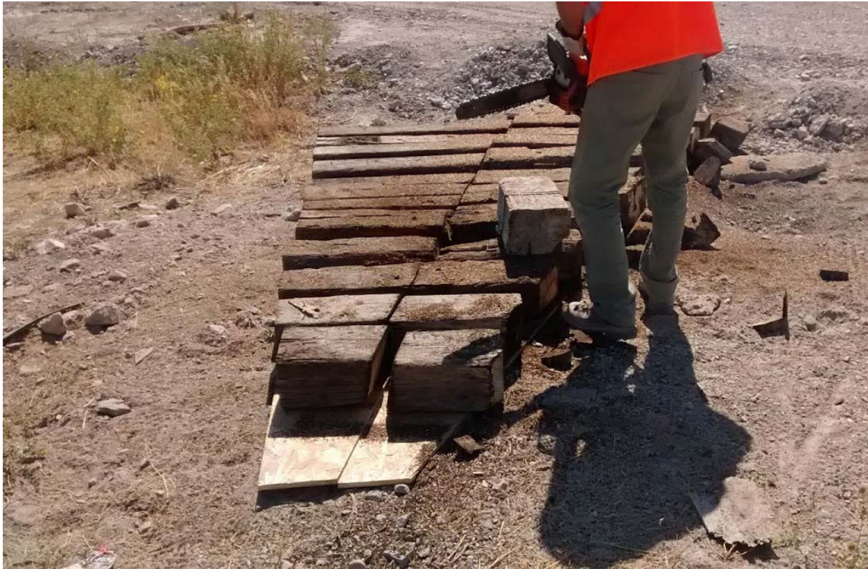
Figure 3-6. Skew wedge base fabrication.
