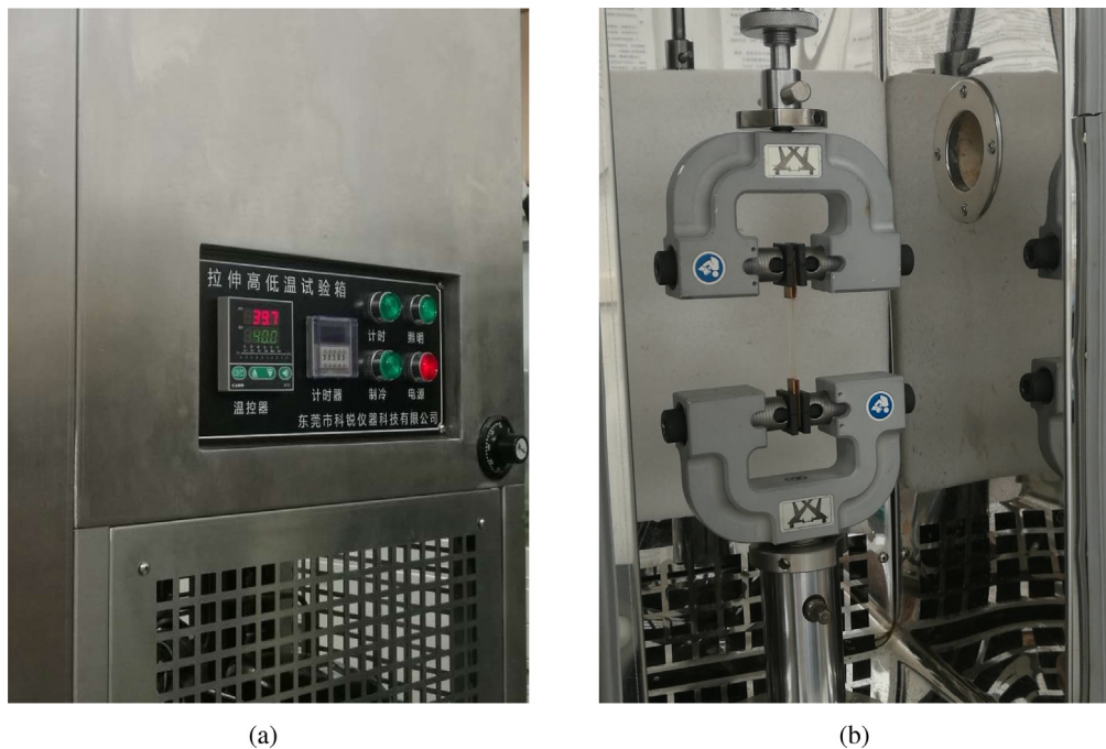
Fig. 3. (a) Temperature monitor device, (b) tensile test preparation equipment.
