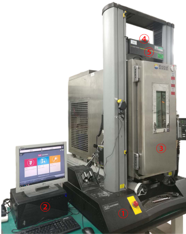
Fig. 2. A complete thermo-viscoelastic testing system: (1) is the main framework of the Instron 5567, (2) is the control computer, (3) is the temperature chamber, (4) is the force transducer to monitor the applied force, and (5) is the crosshead of (1).
