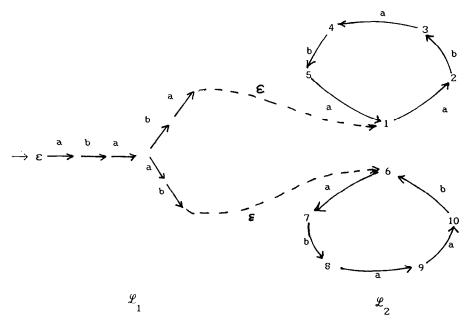
Fig. 4. Automata  $\mathcal{L}_1$ ,  $\mathcal{L}_2$ : the case where x and y are conjugate, x = ababa, y = abaab.
