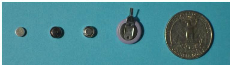
Figure 3.1 Commercial coin cells. (1) ML414 (rechargeable), (2) PR521 (primary), (3) SR527 (primary), and (4) ML1220 (rechargeable) with a quarter dollar (USA).
