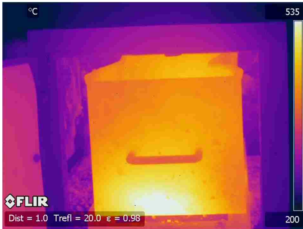
Figure 3.2. Firebox Thermal Image (°C).
