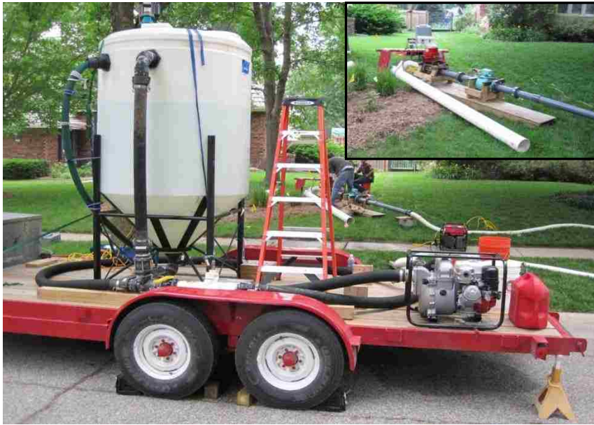
Figure 4. Runoff simulator at site 3. Large image shows water supply tank, trash pump, and trailer hose configuration. Smaller insert image shows magnetic flow meter (blue), control valve (red), and plumbing making up the delivery system at the rain garden inlet.
