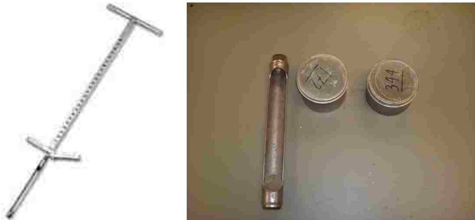
Figure 6. Step soil probe (left). Probe extension and soil tins (right).
