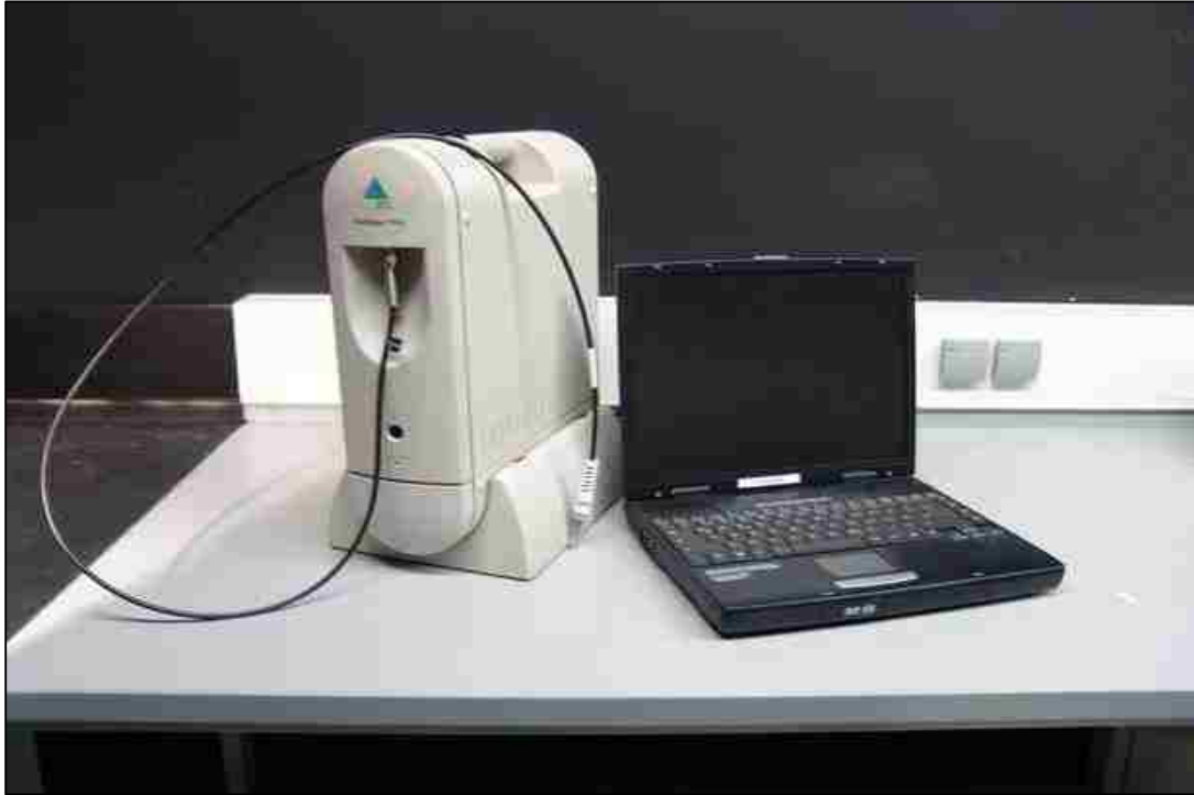
Figure 3.4: FieldSpec-Pro connected with the laptop and ready to use (Source: goo.gl/2TZ08E )
