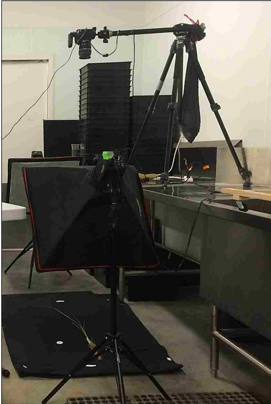
Figure 3.2: Plant imaging setup for D.I.R.T. analysis using Canon EOS 50D camera
