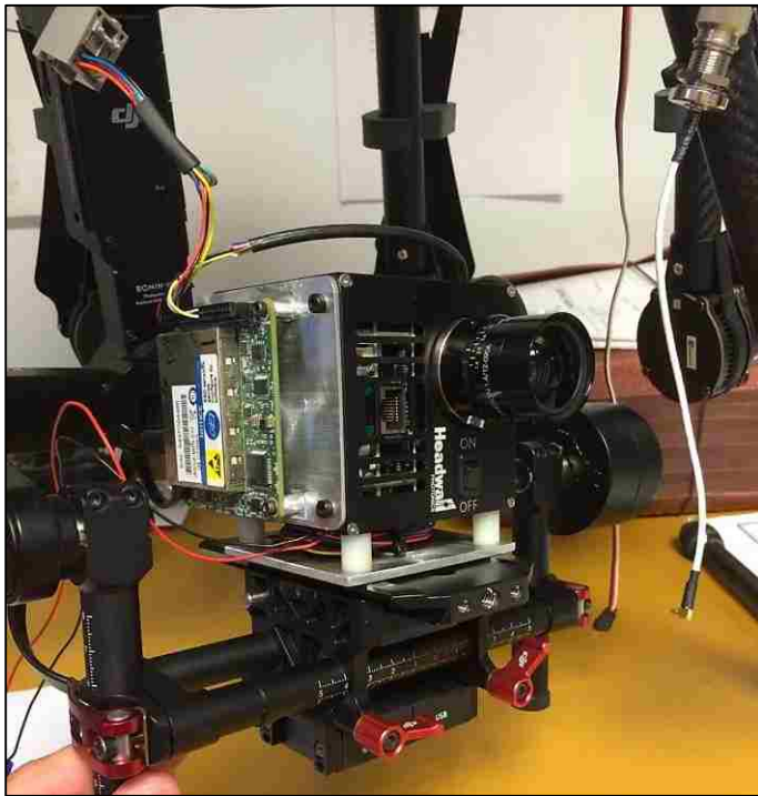
Figure 3.3: Headwall Nano-Hyperspec ® hyperspectral VNIR Imager mounted on a UAV
