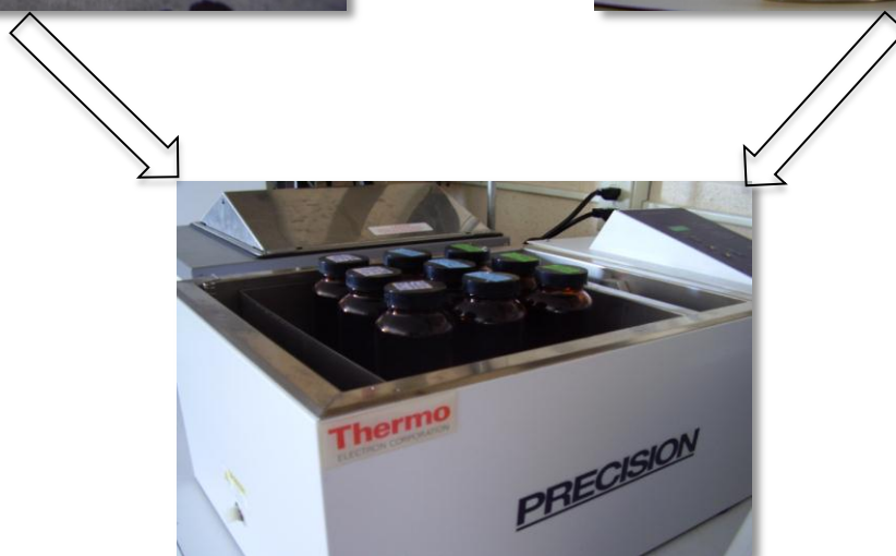
Water bath at 55°C with Amber bottles containing pretreated biomass and enzyme mixture
