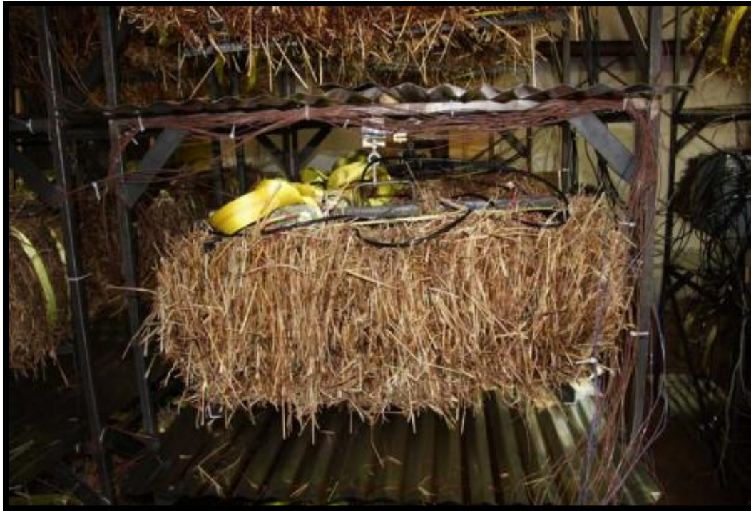
Figure 6: An example of bales hanging on the rack with instrumentation.
