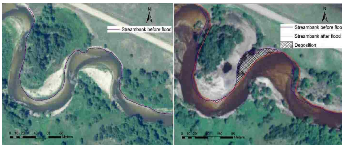
Figure 3.9 A reach on Cedar River illustrating the deposition of sediment in post-flood period (right) compared to pre-flood period (left).
