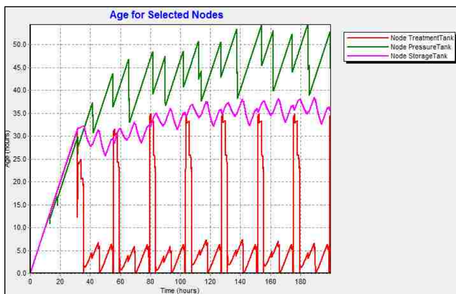
Figure 3.9 Maximum Water Age for the Complex Greywater System with Treatment.
