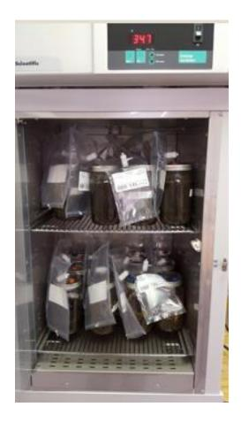
**Figure 1** An image showing the general setup used for the anaerobic digestion batch experiments, in which substrate was placed in jars capped with a lids modified to vent into a Tedlar gas sampling bag and placed in an incubator to be maintained at a temperature of 37°C.
