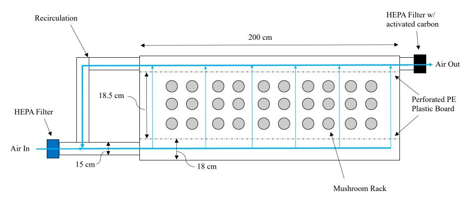
Figure 3 Sketch of mushroom growth chamber that shows dimensions, major components, and air flow.
