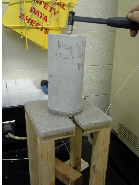
Figure 3-15 Free-free resonant testing.
