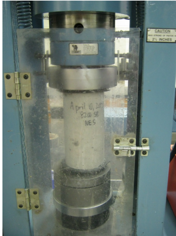
Figure 3-13 Compressive strength testing.
