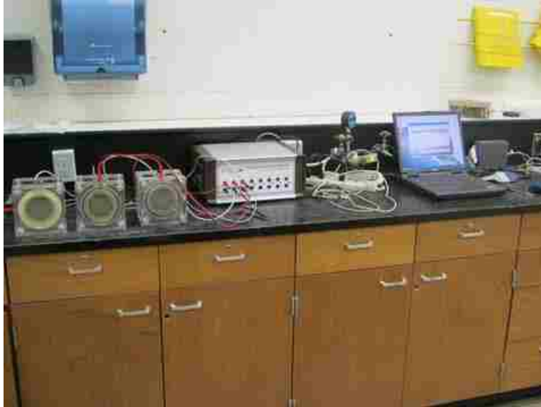
Figure 3-14 Rapid chloride permeability testing.
