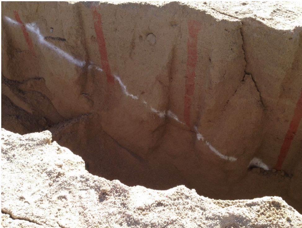
Figure 4.19. Estimate of shear failure surface from four consecutive soil columns.
