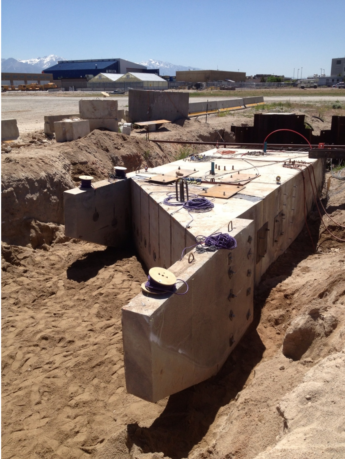
Figure 3.17. Large-scale 45° skewed abutment with reinforced concrete wingwalls.
