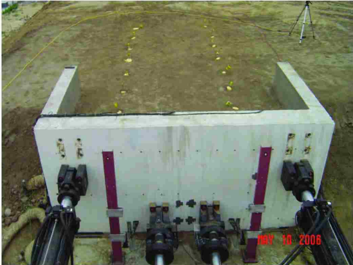
Figure 4.35. Position of applied load (Bozorgzadeh et al. 2008).
