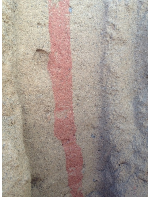
Figure 4.18. Offset in red soil column from shear failure surface.
