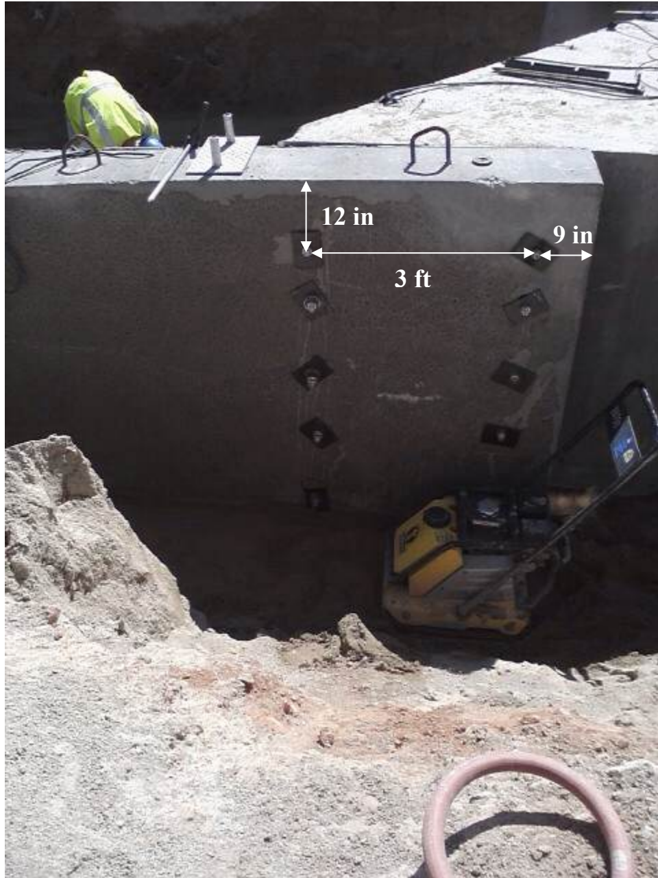
Figure 3.13. Wingwall bolt spacing used for large-scale testing.
