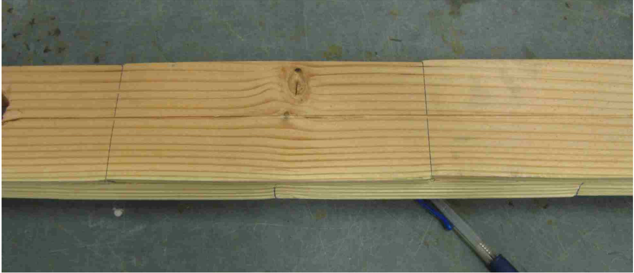
Figure B-3: Dovetail Member Crushing, Marked in Pen (Wall 1).
