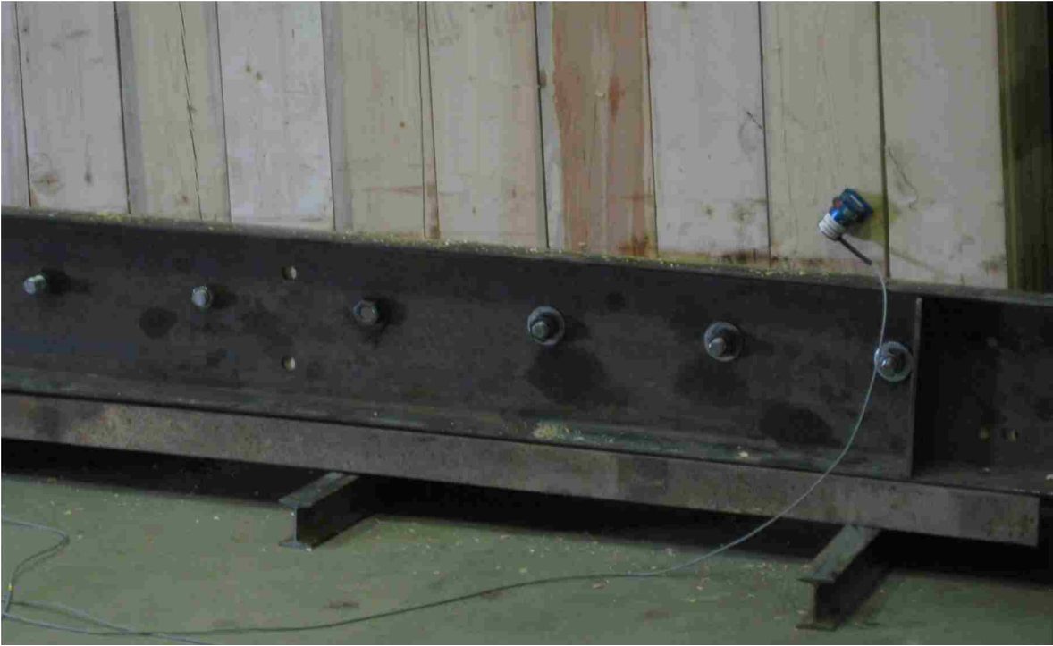
Figure 3-6: Bottom Connection with Additional Channel
