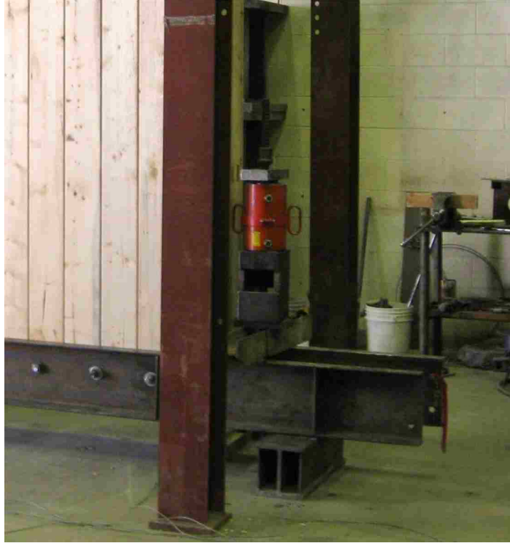
Figure 3-5: Bottom Attachment with Post-Tensioned DYWIDAG
