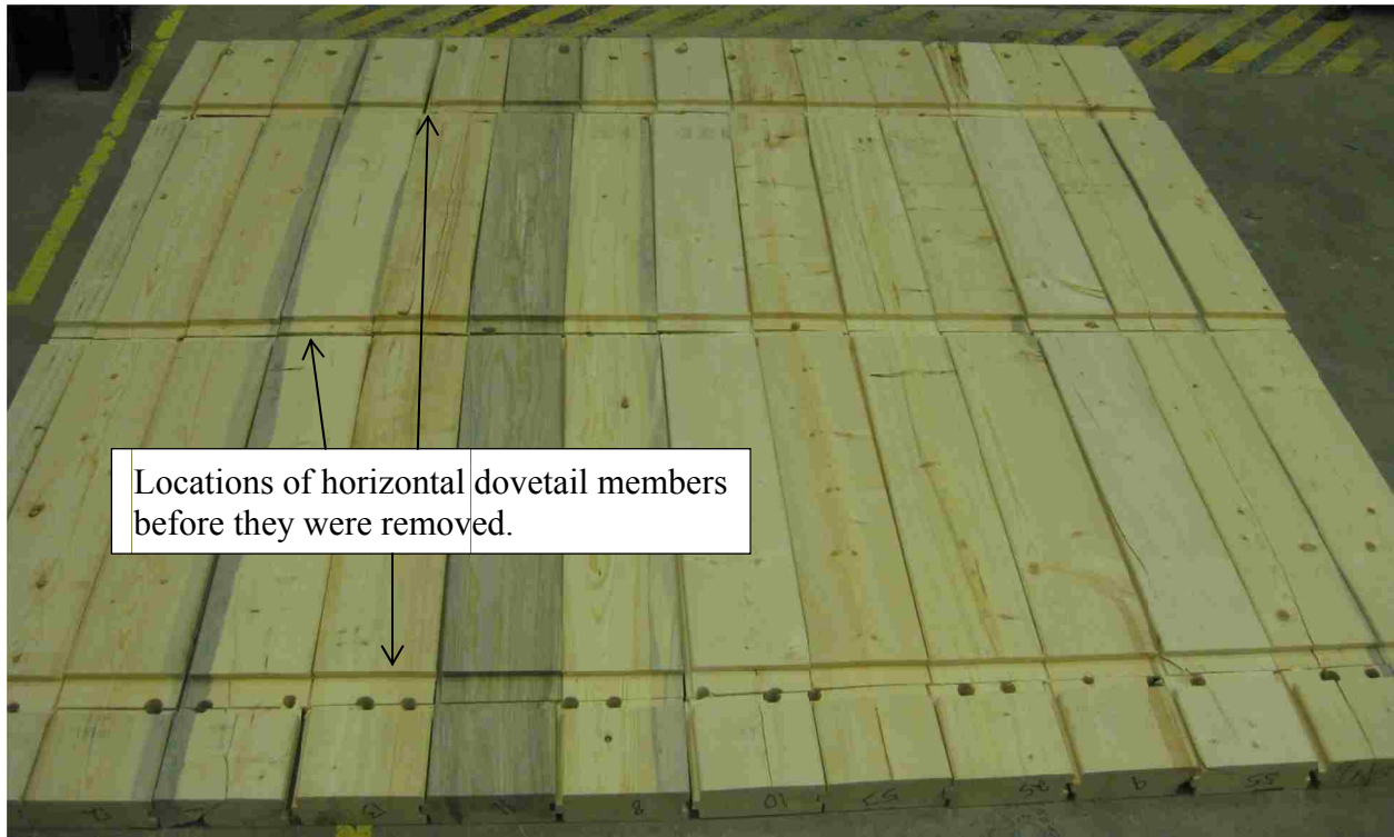
Figure 4-4: First Layer of Vertical Members Removed from the Rest of the Panel After Testing.
