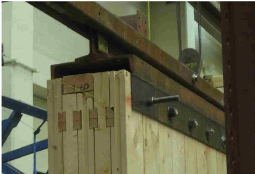
Figure 3-4: Wall to Cap Connection
