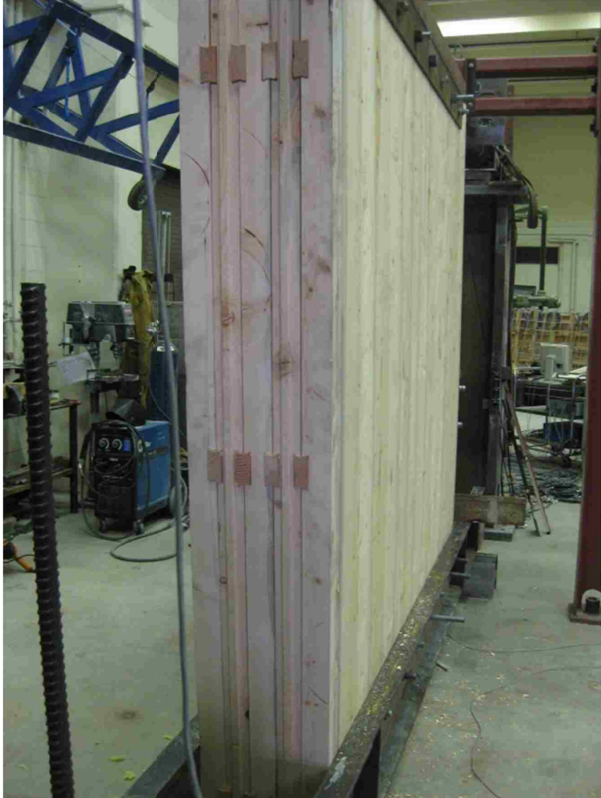
Figure 2-5: Profile View of Type I VOIT Panel
