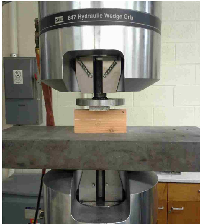
Figure 3-9: Perpendicular to Grain Compression Test
