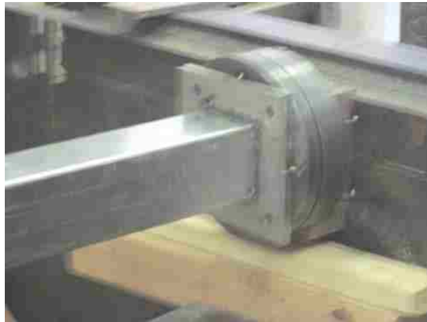
Figure 3-14: Close-up Photo of Boundary Conditions (Reaction-End) During Test to Failure
