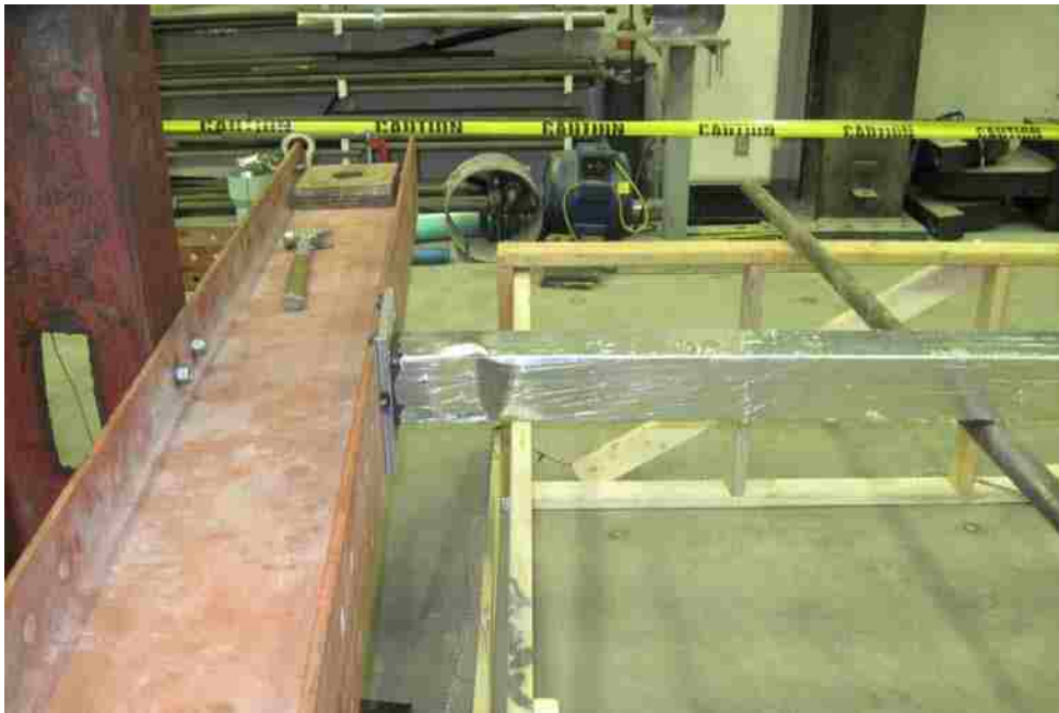
Figure 5-9: Photo of Crippled “Adhesive-No-Foam” Column During Test to Failure
