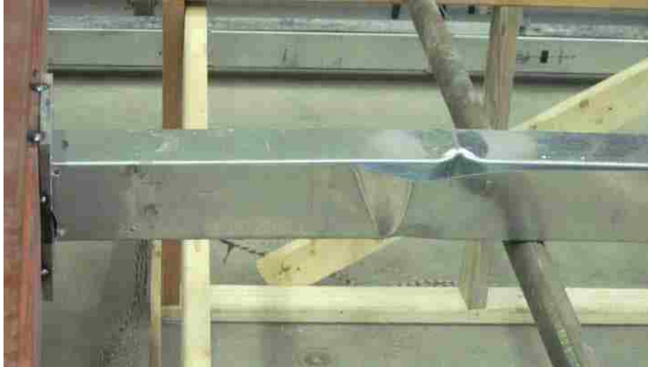
Figure 5-4: Photo of Crippled “Adhesive-Only” Column During Test to Failure
