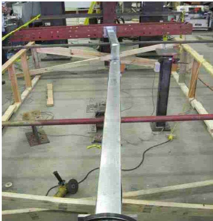
Figure 7-4: Photo of Global Buckling of “Adhesive and Welds” Column During Test to Failure
