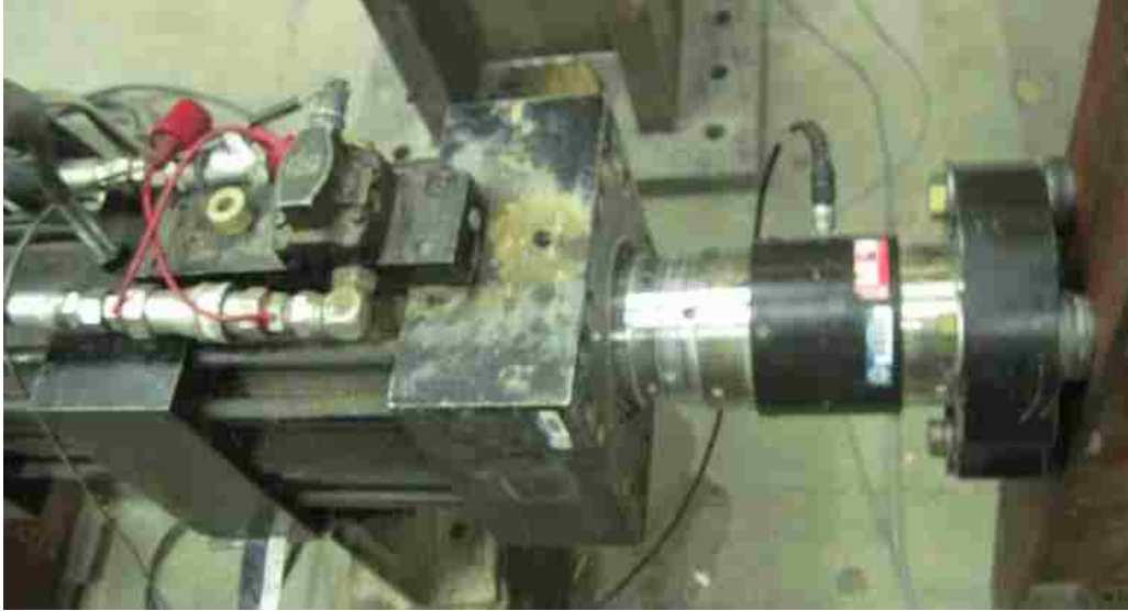
Figure 3-11: Photo of 100-kip Actuator for Tests to Failure
