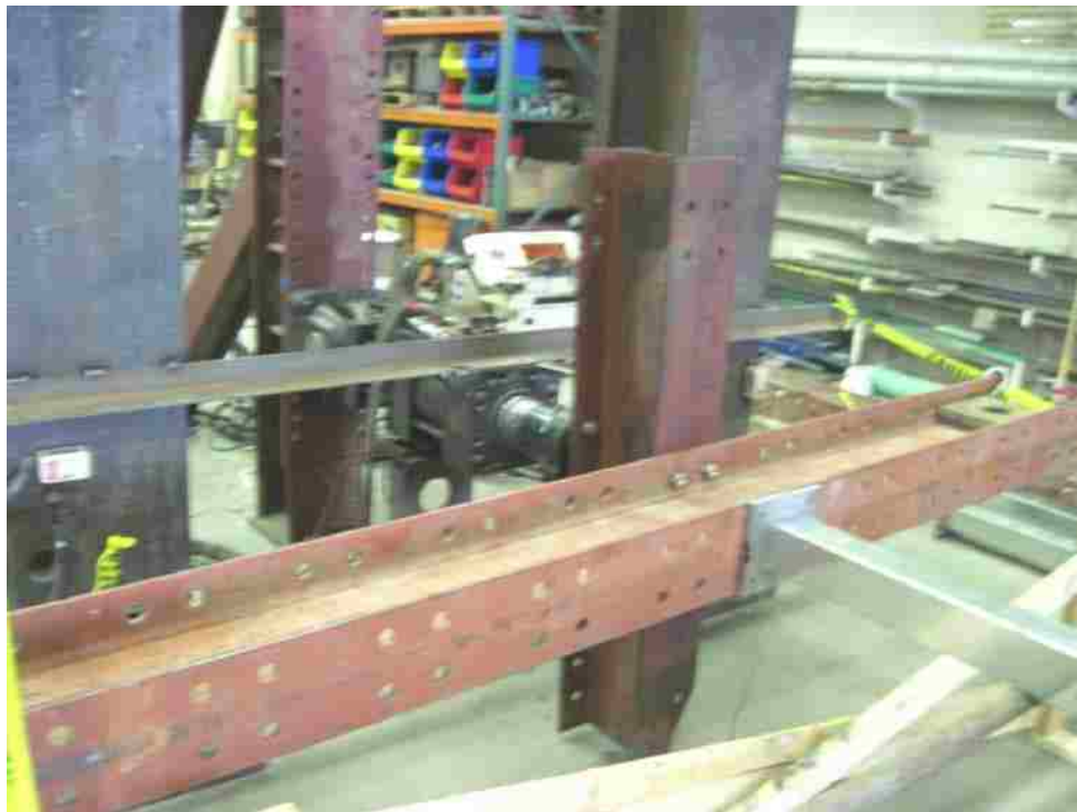
Figure 3-12: Photo of Boundary Conditions (Actuator-End) During Test to Failure
