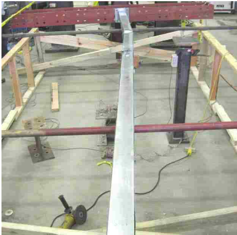
Figure 5-5: Photo of Buckled “Adhesive and Welds” Column During Test to Failure
