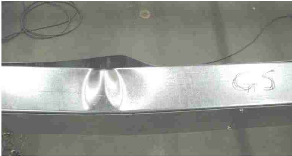
Figure 5-8: Close-up Photo of Crippling of “Adhesive and Screws” Column During Test to Failure
