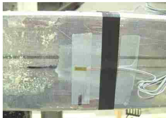
Figure 3-18: Close-up Photo of Mid-Span Strain Gage on Column Tested to Failure
