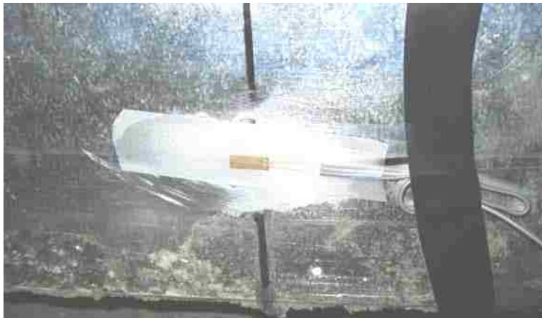
Figure 3-8: Photo of Typical Strain Gage Attachment for Test to 20 kips
