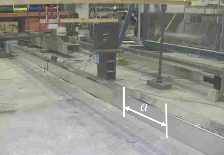
Figure 4-1: Photo of Local Buckling in “Adhesive-Only” Column During Test to 20 kips Showing Local Buckling Wavelength
