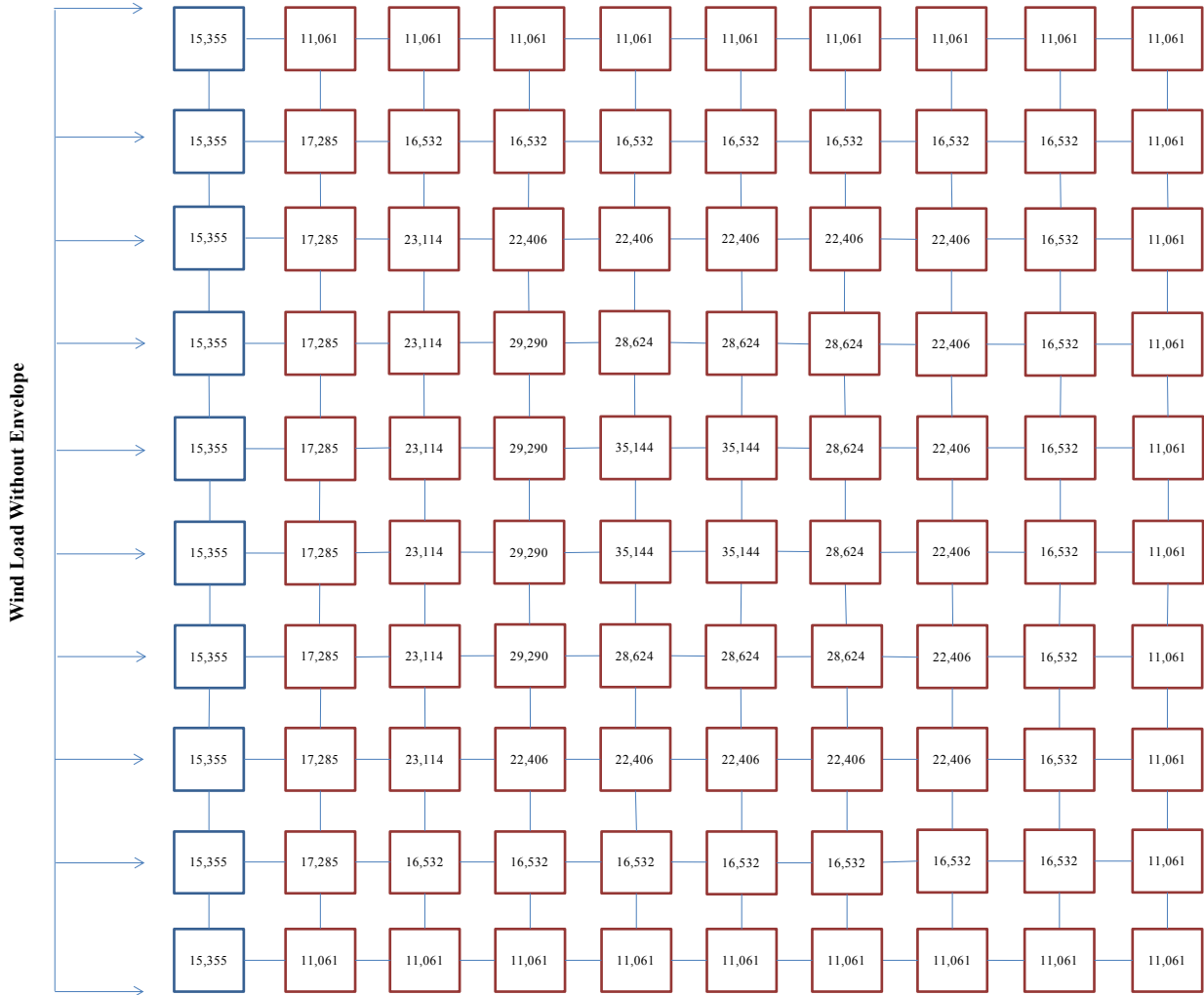
Figure 5-19: Total Lateral Wind Loads for 100-Skyscraper Pyramid Without Envelope
