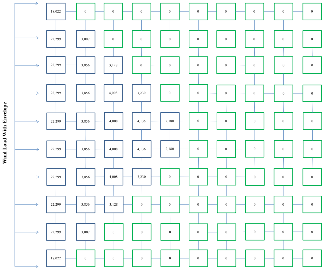
Figure 5-18: Total Lateral Wind Loads for 100-Skyscraper Pyramid With Envelope
