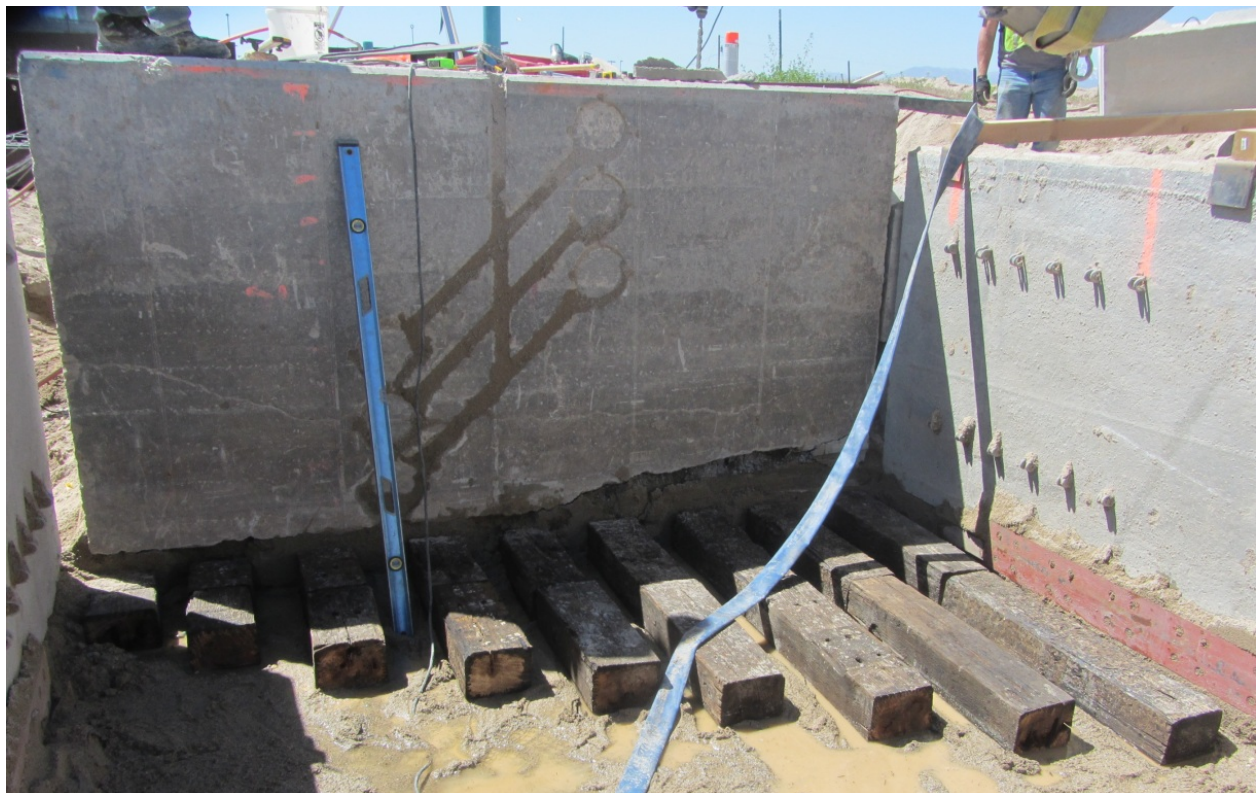
Figure 3-9: Railroad tie foundation for 15° and 30° wedges
