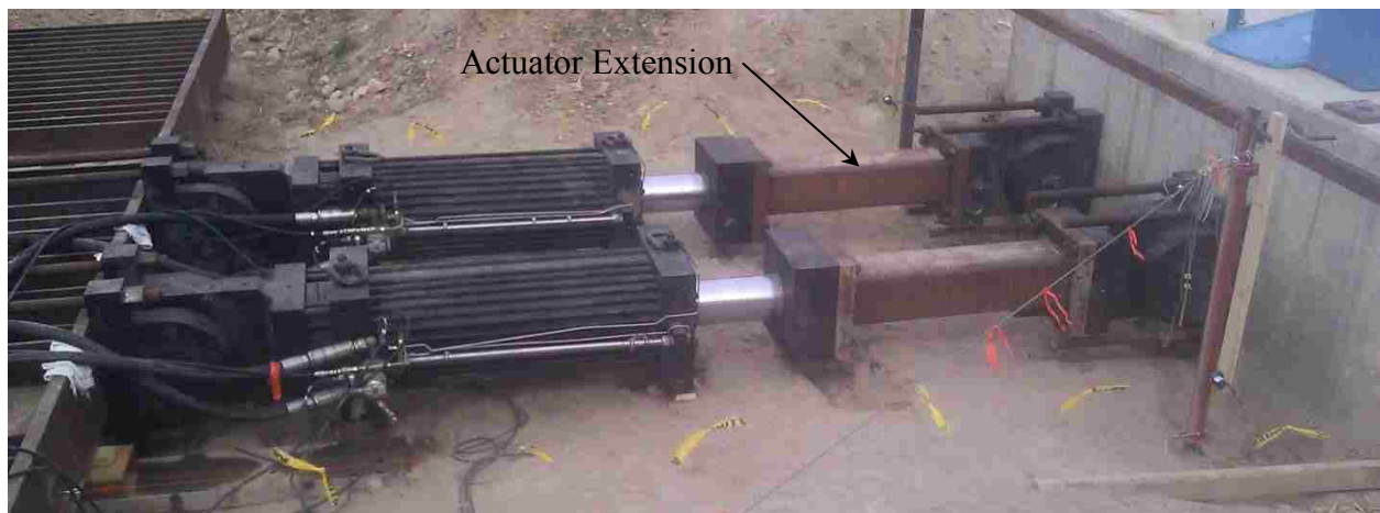
Figure 3-13: MTS hydraulic actuators
