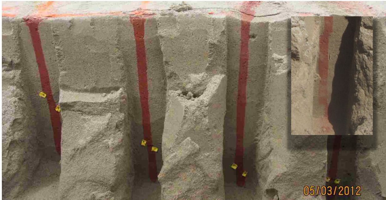
Figure 3-18: Offset in red sand columns showing upper failure surface of the 0° test (inset more clearly shows column offset at test completion)
