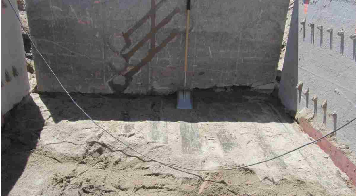
Figure 3-9: Railroad tie foundation for 15° and 30° wedges with sand compacted between ties (Marsh, 2013)
