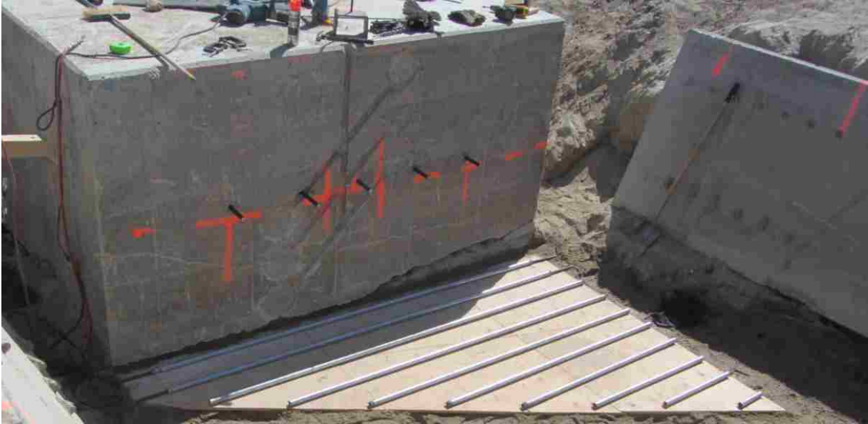
Figure 3-10: Roller foundation for 15° and 30° wedges (Marsh, 2013)
