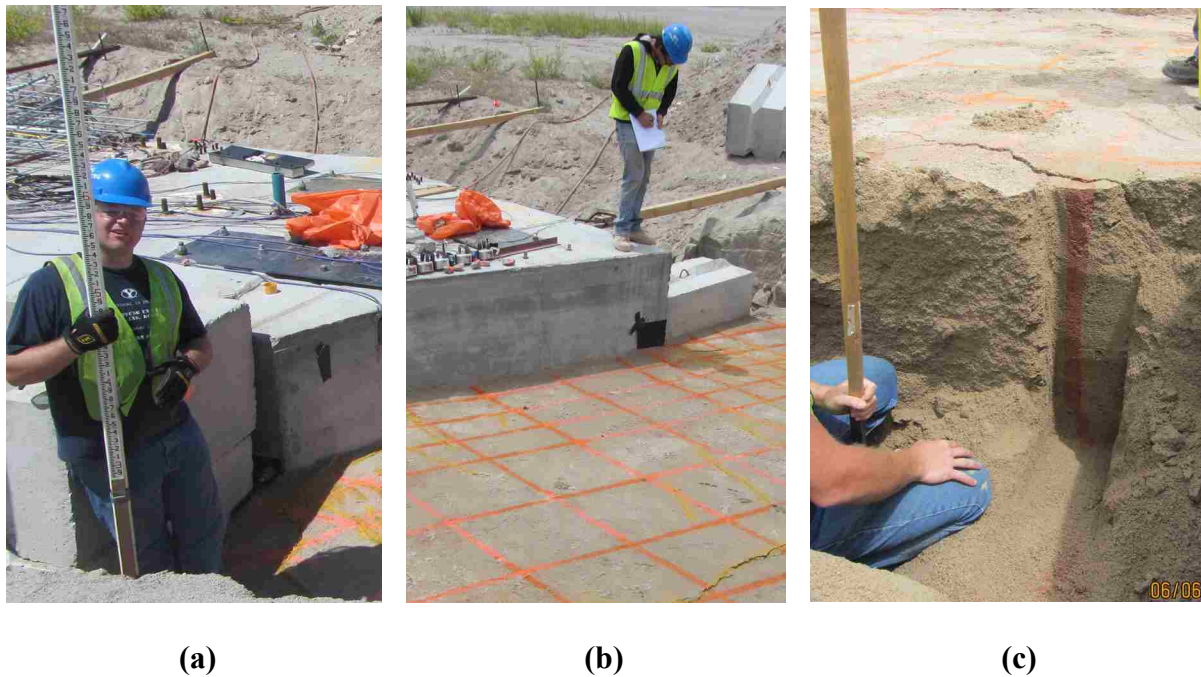
Figure 3-35: Post-testing recordings including (a) backfill heave elevation, (b) mapping of developed soil cracks, and (c) shear failure locations within red sand columns
