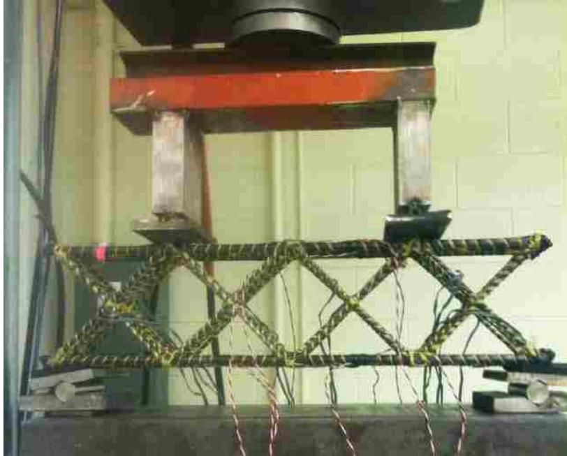
Figure 2-11: Picture of Four-Point Bending Test Setup
