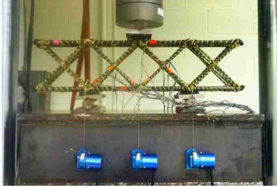
Figure 2-13: Picture of Three-Point Bending Test Setup
