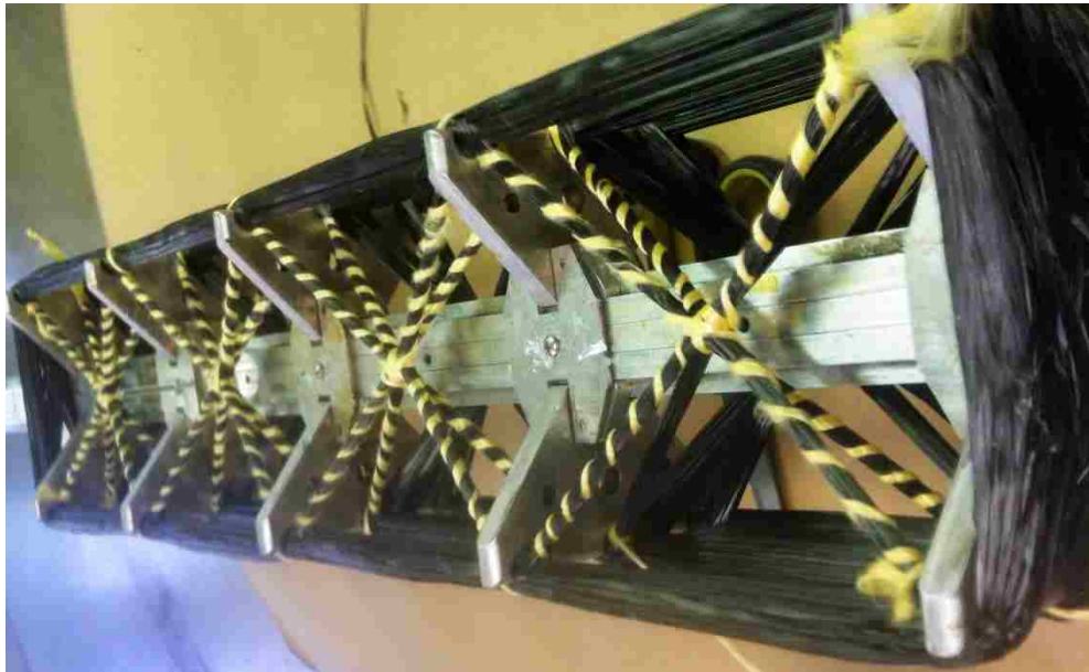
Figure 2-2: Picture of Inner Diagonal Consolidation
