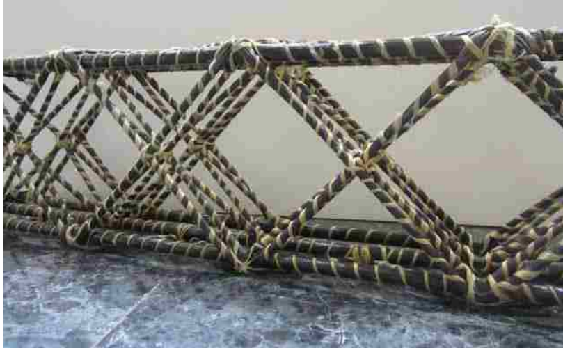
Figure 1-5: Picture of IsoBeam Test Specimen
