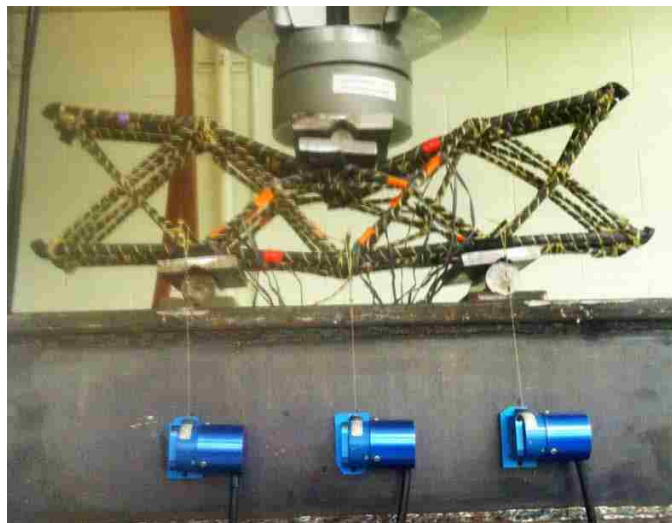
Figure 7-3: IsoBeam Specimen at 25% of Peak Loading
