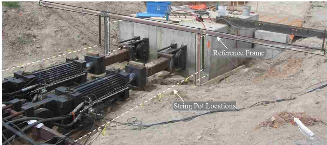
Figure 3.23: String pot locations and reference frame
