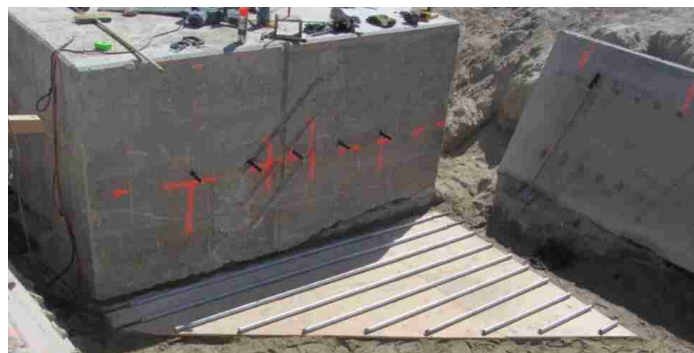
Figure 3.11: Roller foundation for 15° and 30° wedges (Marsh 2013)
