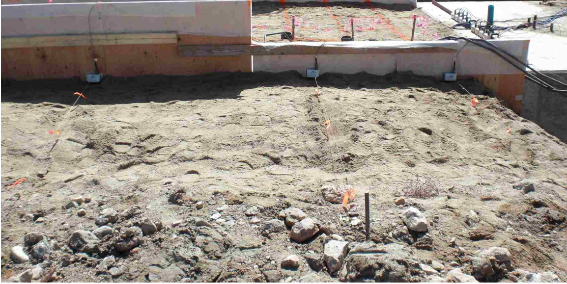
Figure 4-10: String pots on side isolation panels.
