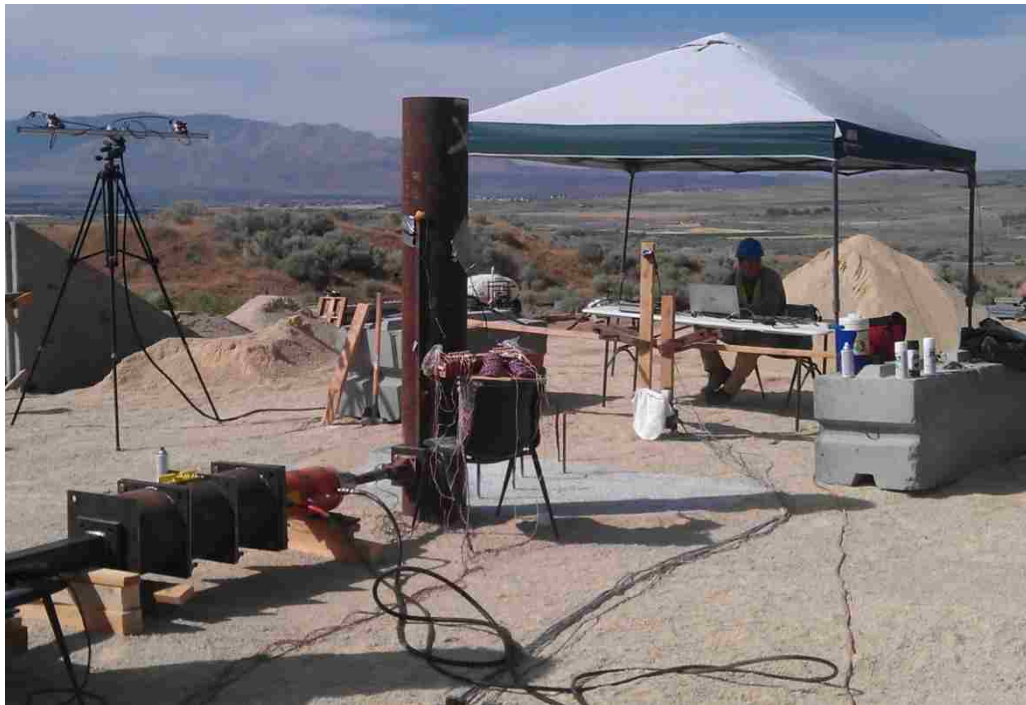
Figure 4-4: Typical DIC Set Up
