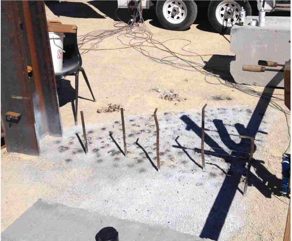
Figure 4-5: Ground Contrast Pattern for DIC Capture
