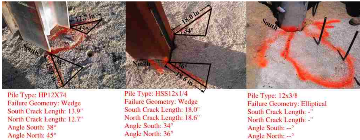
Figure 5-13: Failure Planes for the Distinct Shapes
