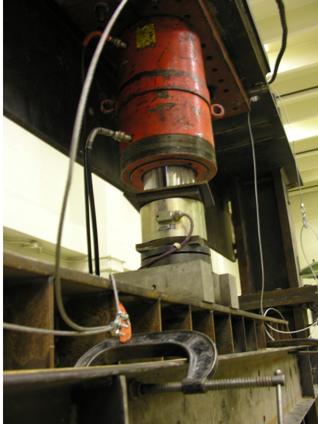
Figure C-3: Hydraulic Jack and Loading Frame of Compression Wall
