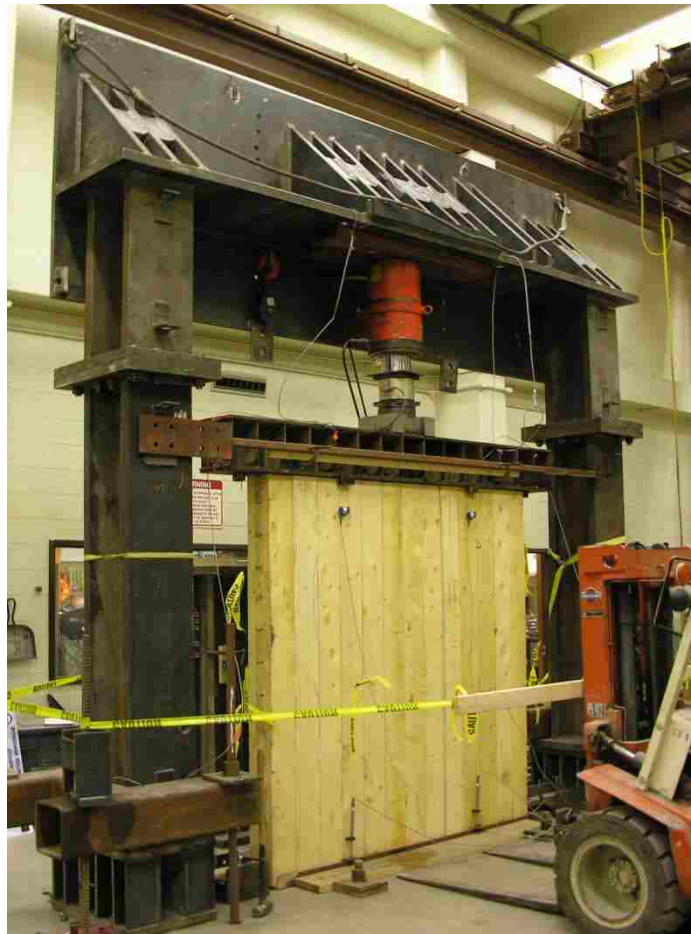
Figure C-1: North Face of Compression Wall Test Setup
