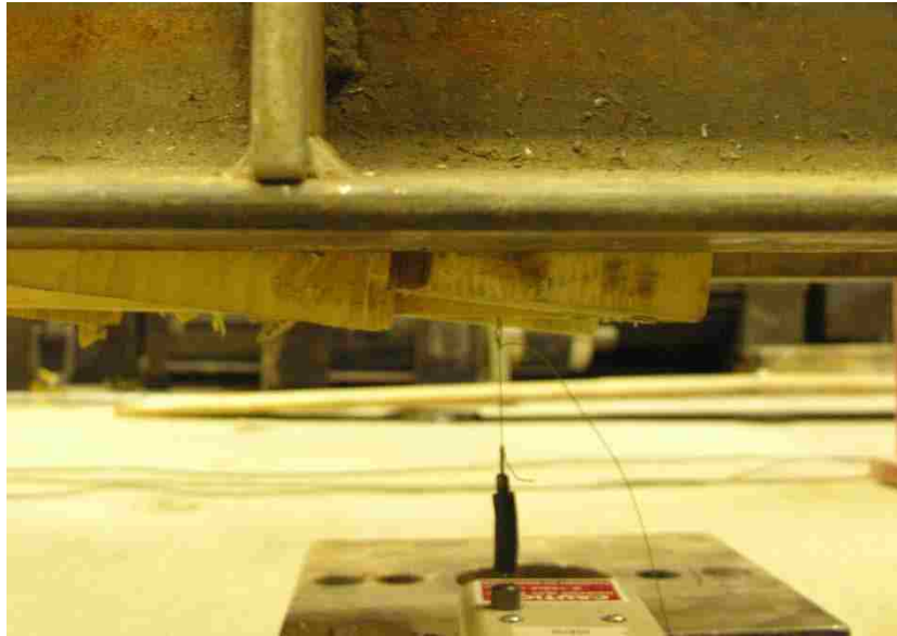
Figure A-3: Vertical Displacement of Racking Wall, East Side
