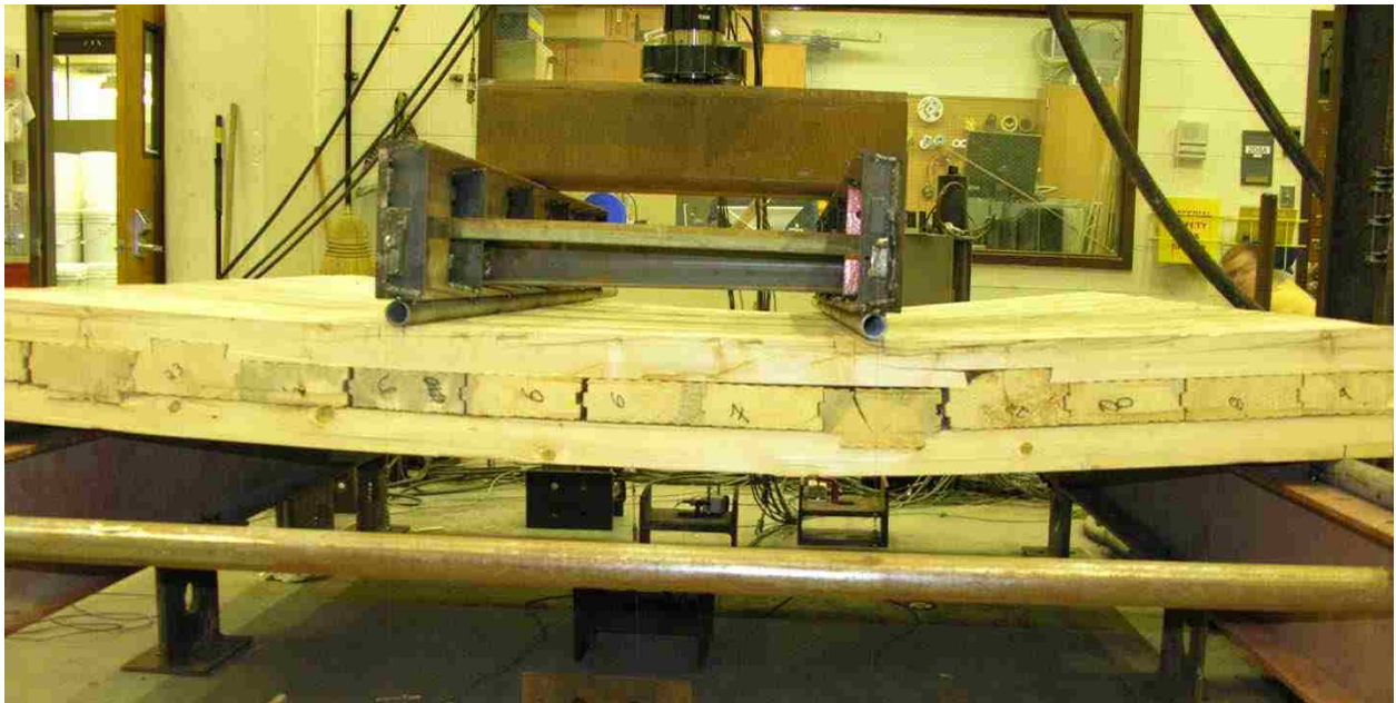
Figure B-3: Failure of Flexural Wall on the North Side
