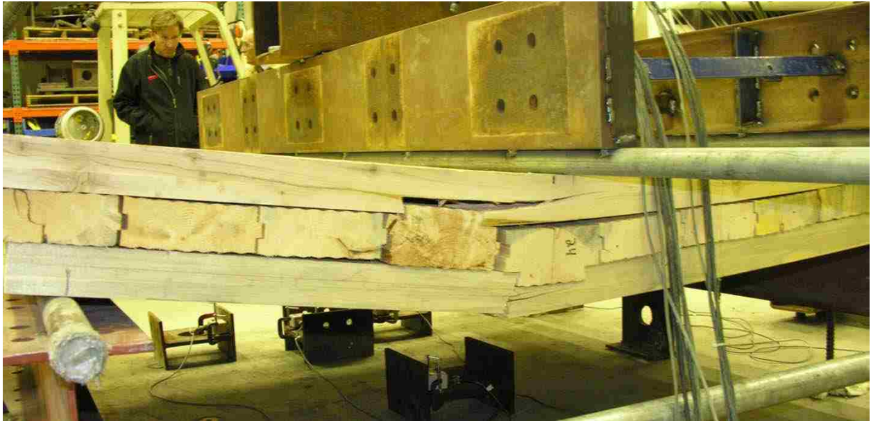
Figure B-4: Failure of Flexural Wall on the South Side
