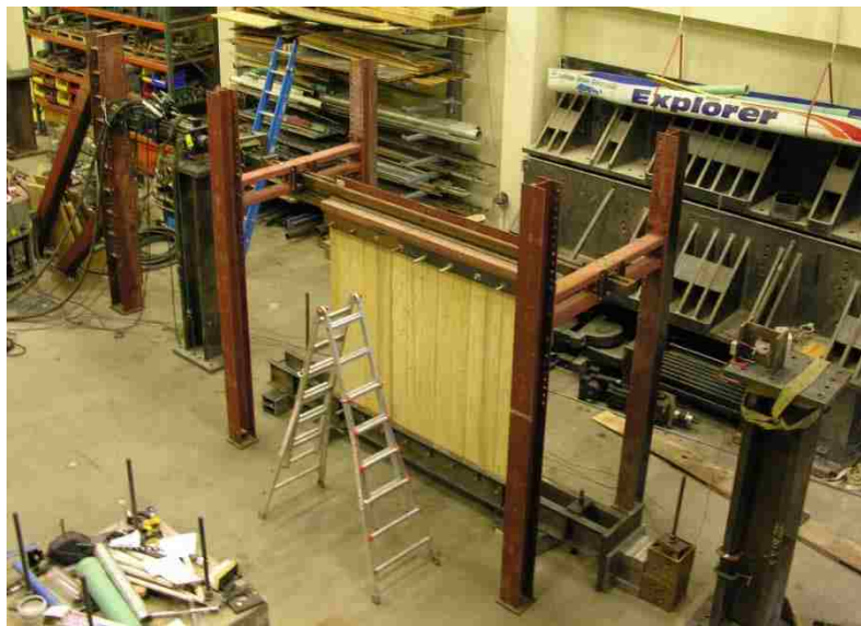
Figure 3-1: In-Plane Lateral Load Test Frame and Setup with an ICLT Wall in Place
