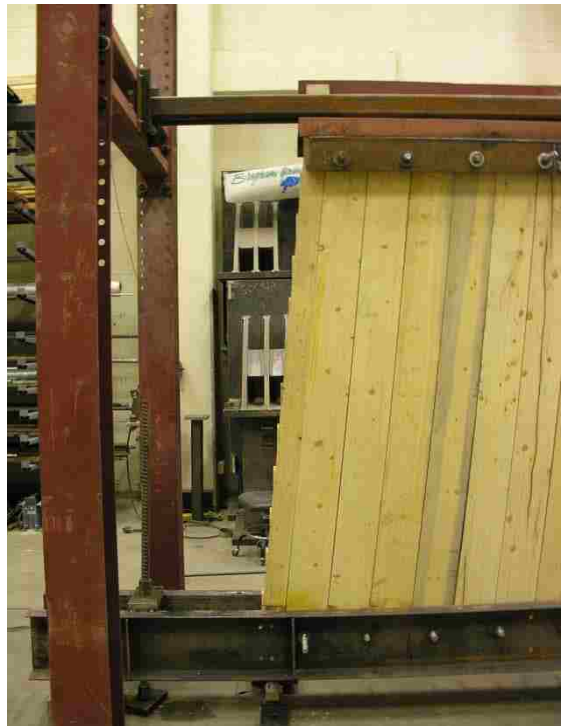
Figure A-2: Lateral Displacement of Racking Wall at Tests Limit
