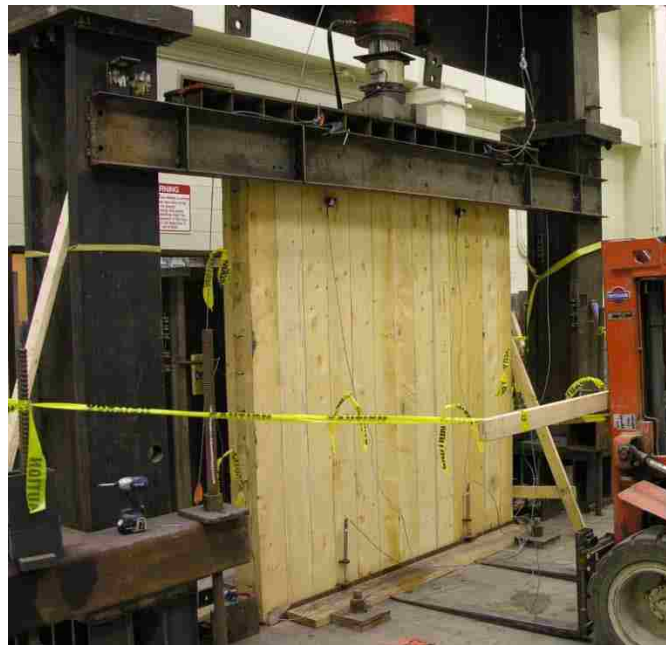
Figure 3-5: In-Plane Vertical Load Test Setup with an ICLT Wall in Place
