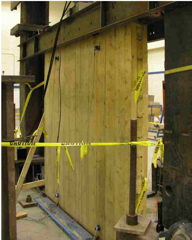
Figure C-2: South Face of Compression Wall Test Setup
