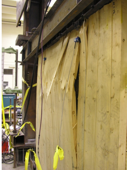
Figure 4-6: Fracture of the In-Plane Vertical Load Test
