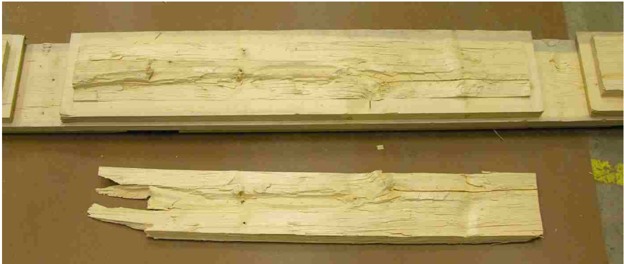
Figure 4-7: Fracture of Horizontal Dovetail Member, In-Plane Vertical Loading Test
