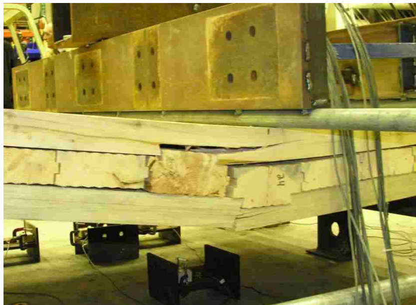
Figure 4-5: Region of Failure at the Out-of-Plane Loading Test.
