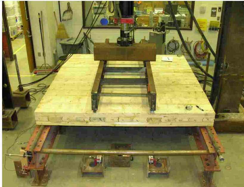
Figure B-1: Flexural Wall Test Setup Looking to the South
