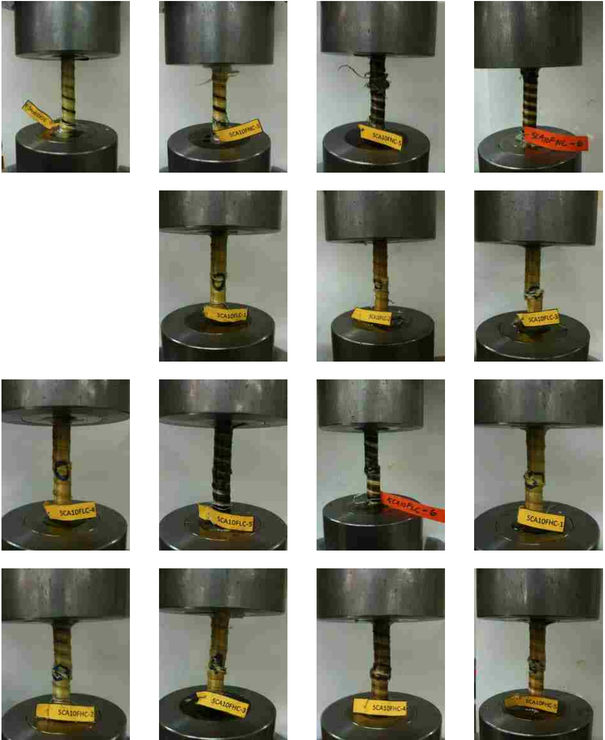
Figure B.3: Pictures of Full Spiral Carbon Specimens After Failure
