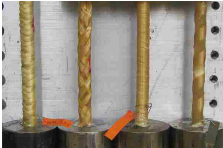
Figure 2.1: Sleeve Configurations from Left to Right: Full Braid, Half Braid, Full Spiral, and Half Spiral
