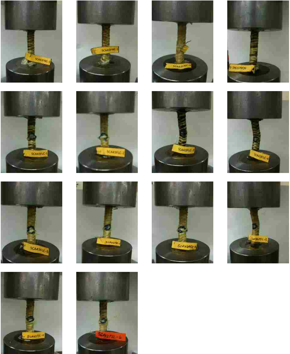
Figure B.1: Pictures of Full Braid Carbon Specimens After Failure
