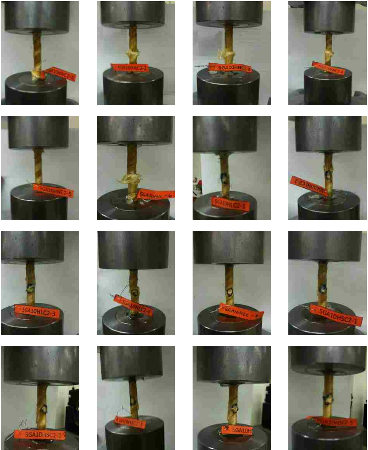
Figure B.8: Pictures of Half Spiral Fiberglass Specimens After Failure
