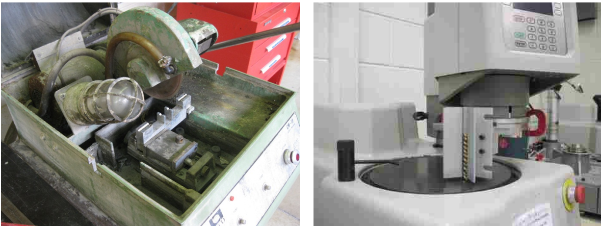
Figure 2.3: Specimen Preparation Equipment: A) Cutting Jig with Diamond Tip Blade (Left); and, B) Polisher with Vertical Aligning Attachment (Right)
