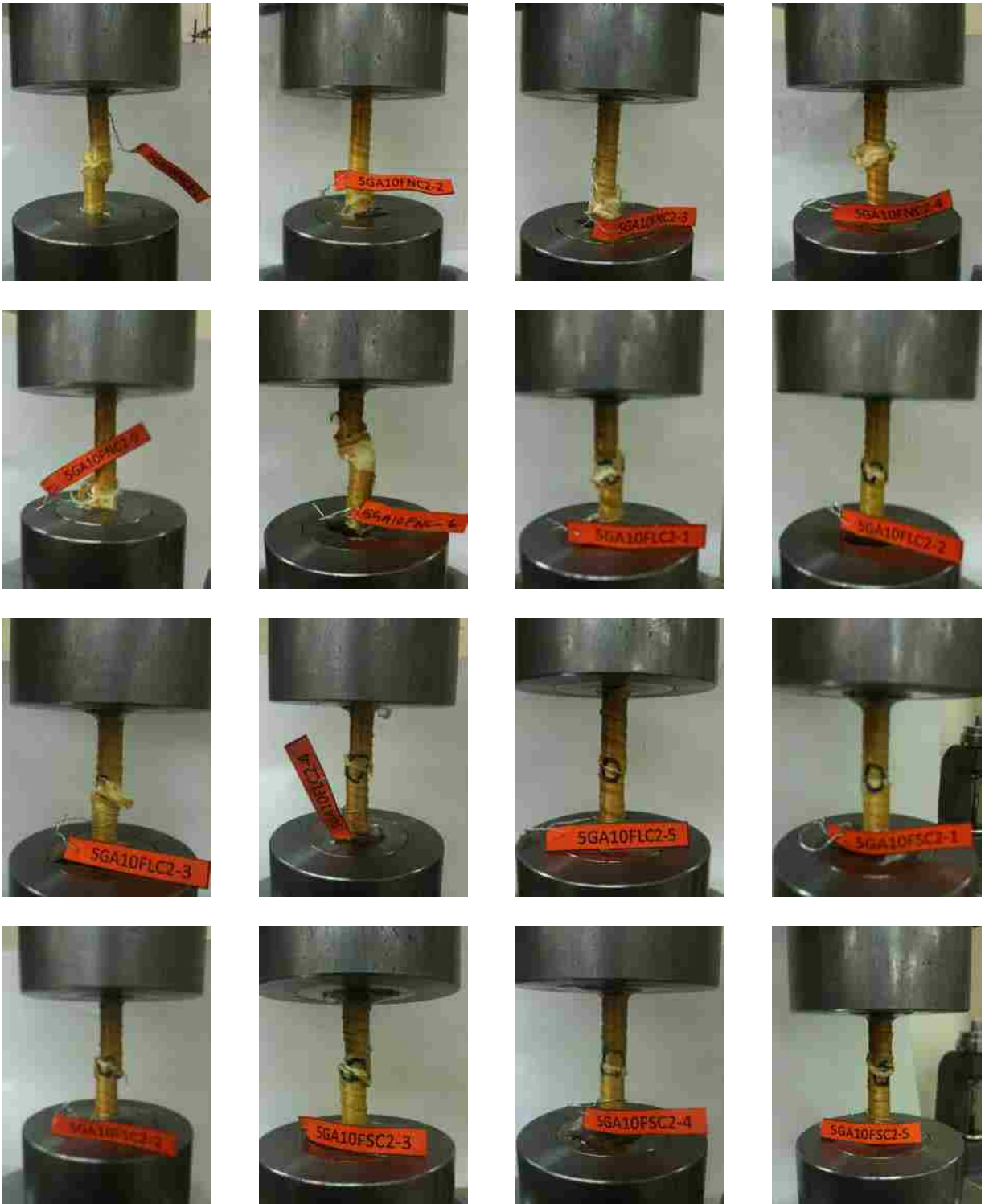
Figure B.7: Pictures of Full Spiral Fiberglass Specimens After Failure
