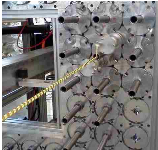
Figure 2.2: Test Specimen Being Fabricated on Prototype IsoTruss Machine
