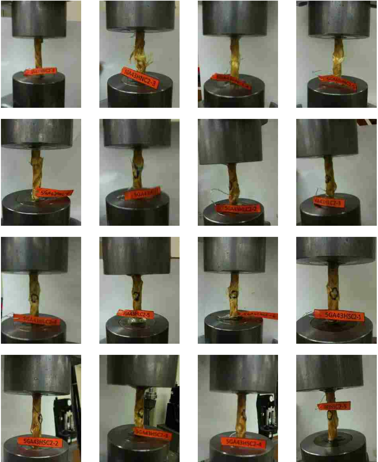
Figure B.6: Pictures of Half Braid Fiberglass Specimens After Failure
