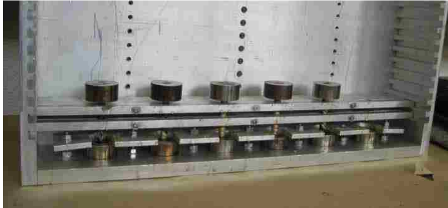
Figure 2.4: Vertical Aligning Fixture used to Bond Specimens in End Caps
