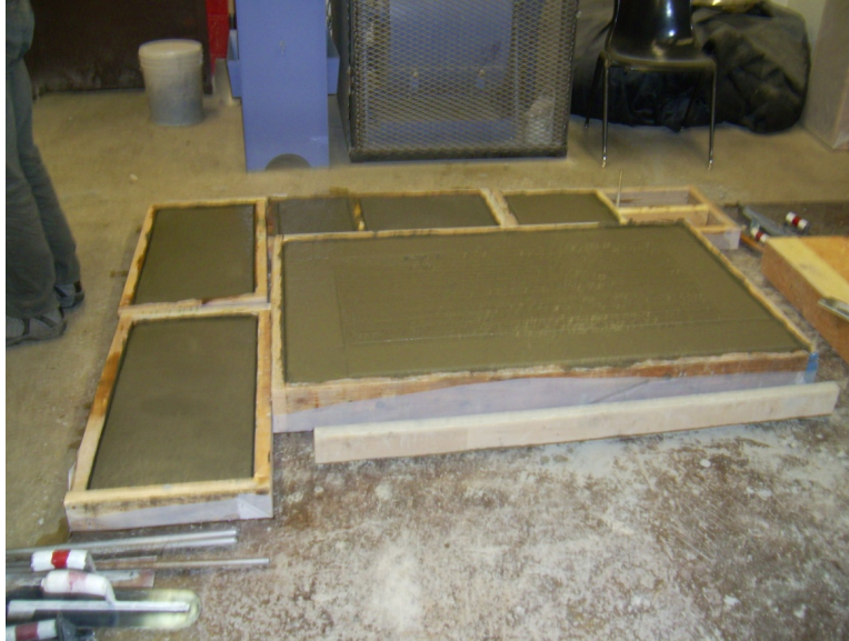
Figure 3-5: Experimental slabs after casting.
