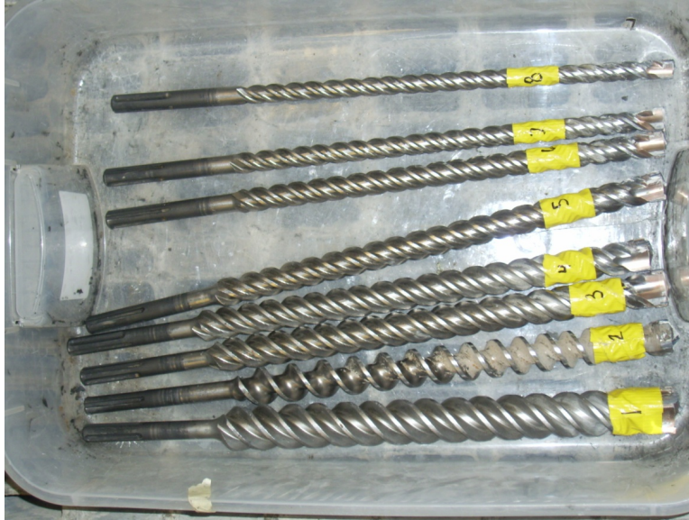
Figure 3-9: Drill bits for stepwise drilling method.
