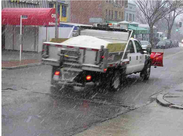
Figure 2-2: Typical deicing salt application.
