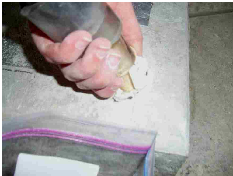
Figure 3-14: Vacuum collection method.
