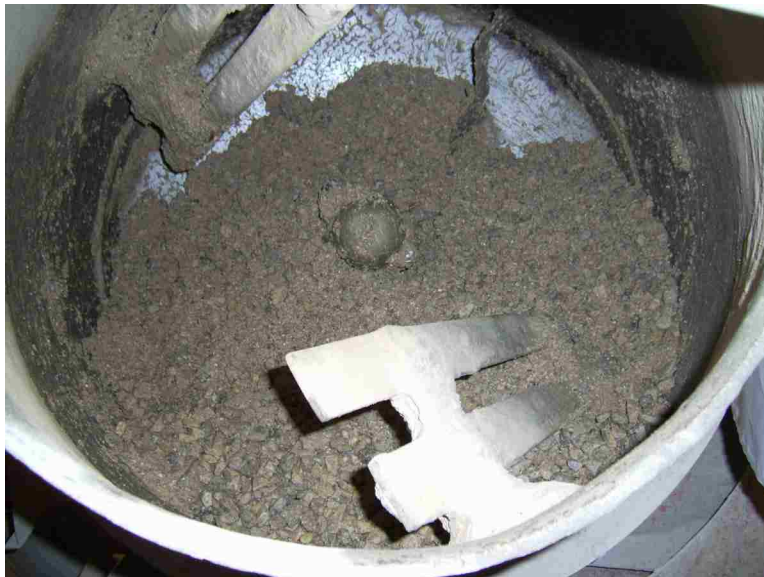
Figure 3-2: Aggregates and water in concrete mixer.
