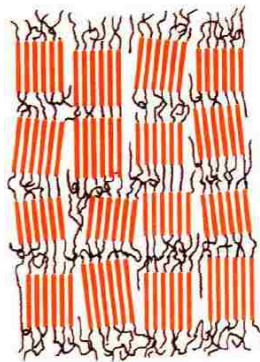
Figure 11: Crystalline Structure Aligning with the Direction of Loading
