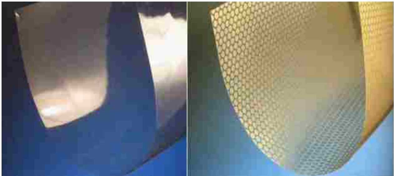
Figure 14: Clear ETFE Foil (left), Reflective Pattern Printed on ETFE Foil (right)
