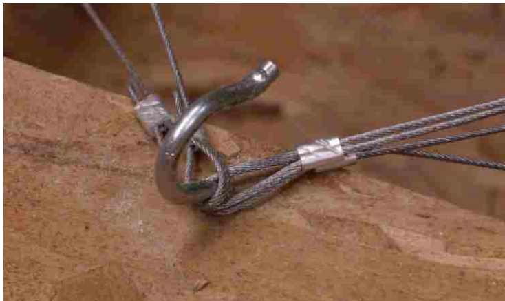
Figure 101: Close Up of Cable Attachments
