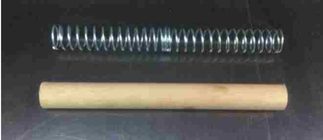
Figure 102: Dowels Used to Replace Springs
