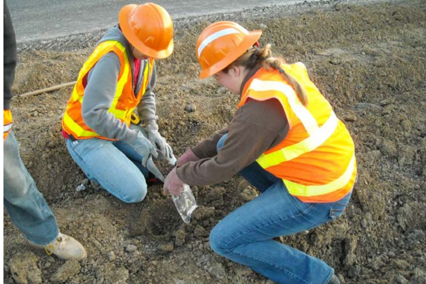
Figure 3-9: Pre-treatment material sampling.
