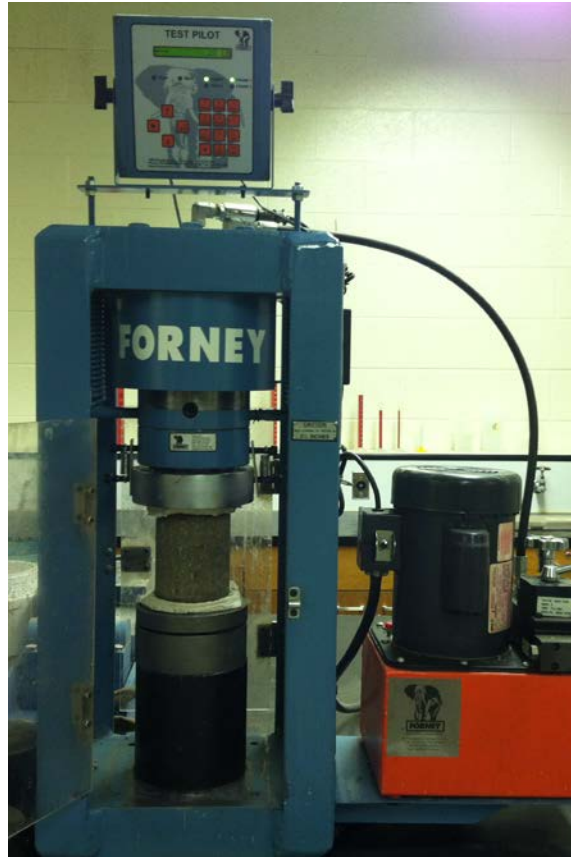
Figure 3-12: Unconfined compressive strength testing.
