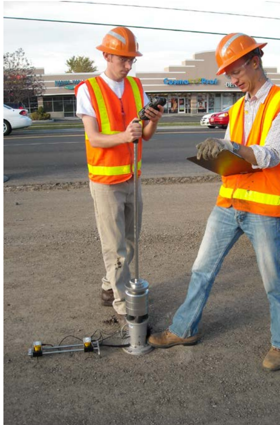
Figure 3-4: Portable falling-weight deflectometer.
