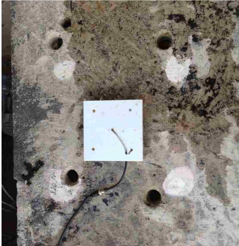
Figure 3-12. Probe placement for slabs in set E.
