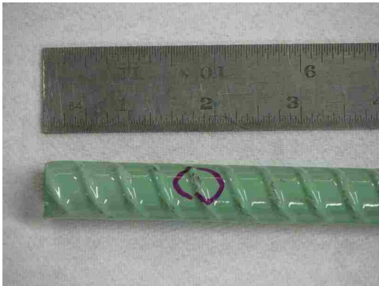
Figure 3-3. Epoxy coating damage from pliers strike.
