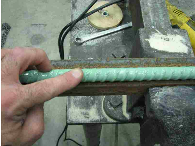
Figure 3-4. Epoxy coating damage from rib scrape.
