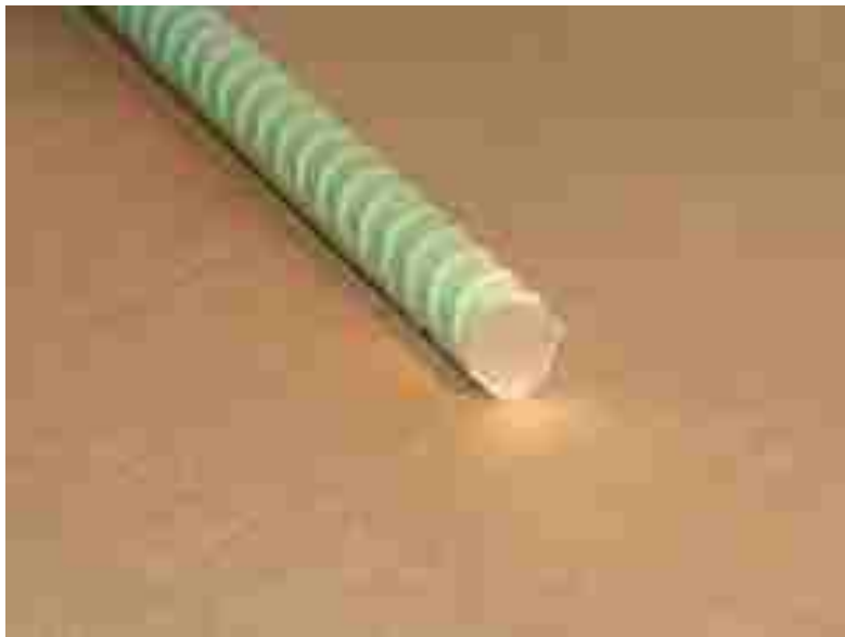
Figure 3-2. Epoxy coating damage from end cut.
