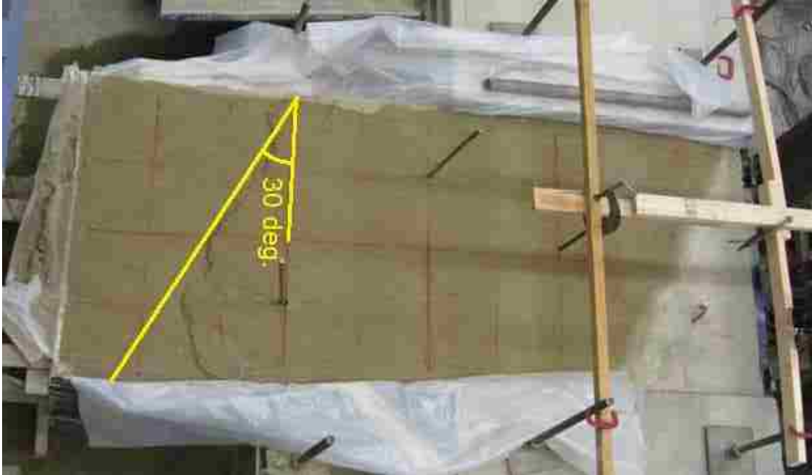
Figure 4-13: Photograph Showing Failure Surface Geometry at Ground Surface for 30° Skew Test
