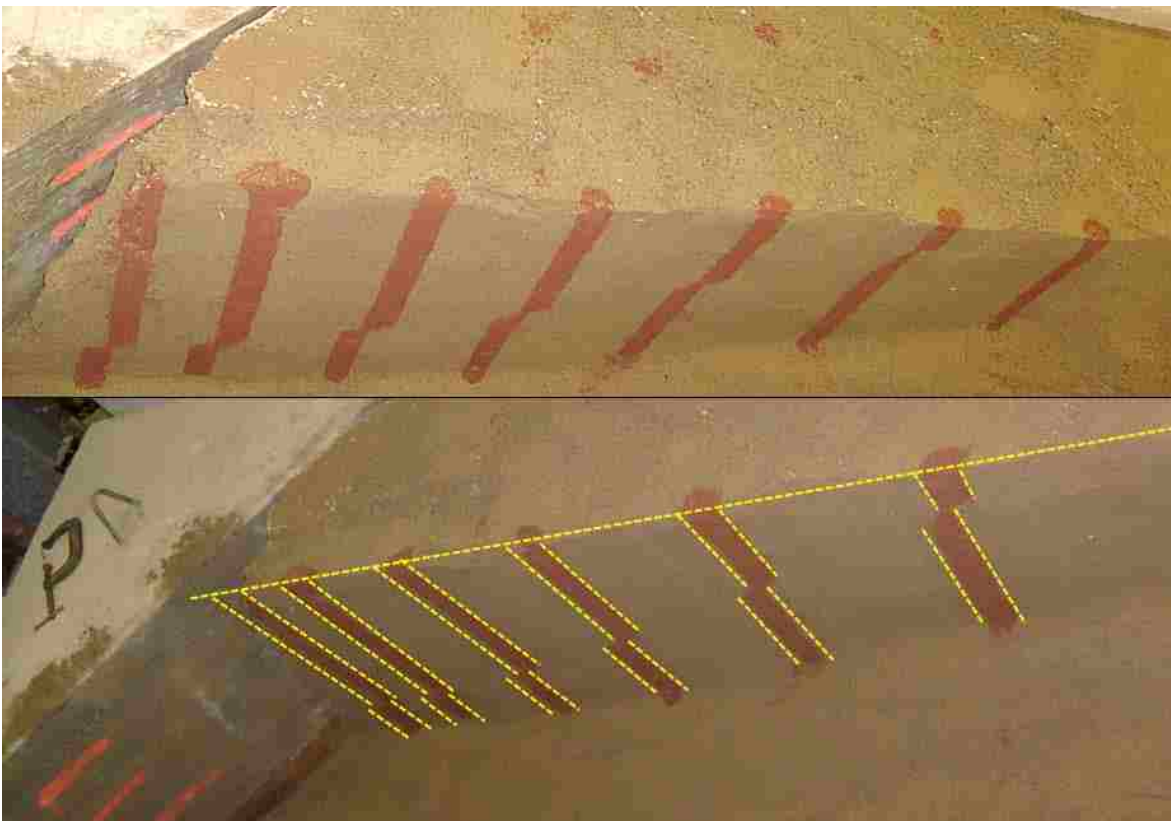
Figure 4-14: Photographs Showing Failure Surface Geometry Within Sand Based on Offset in Red Sand Columns for 45° Skew Test
