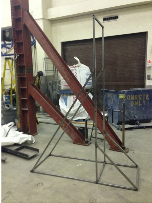
Figure 2-6: Finished steel frame to support three monitors.
